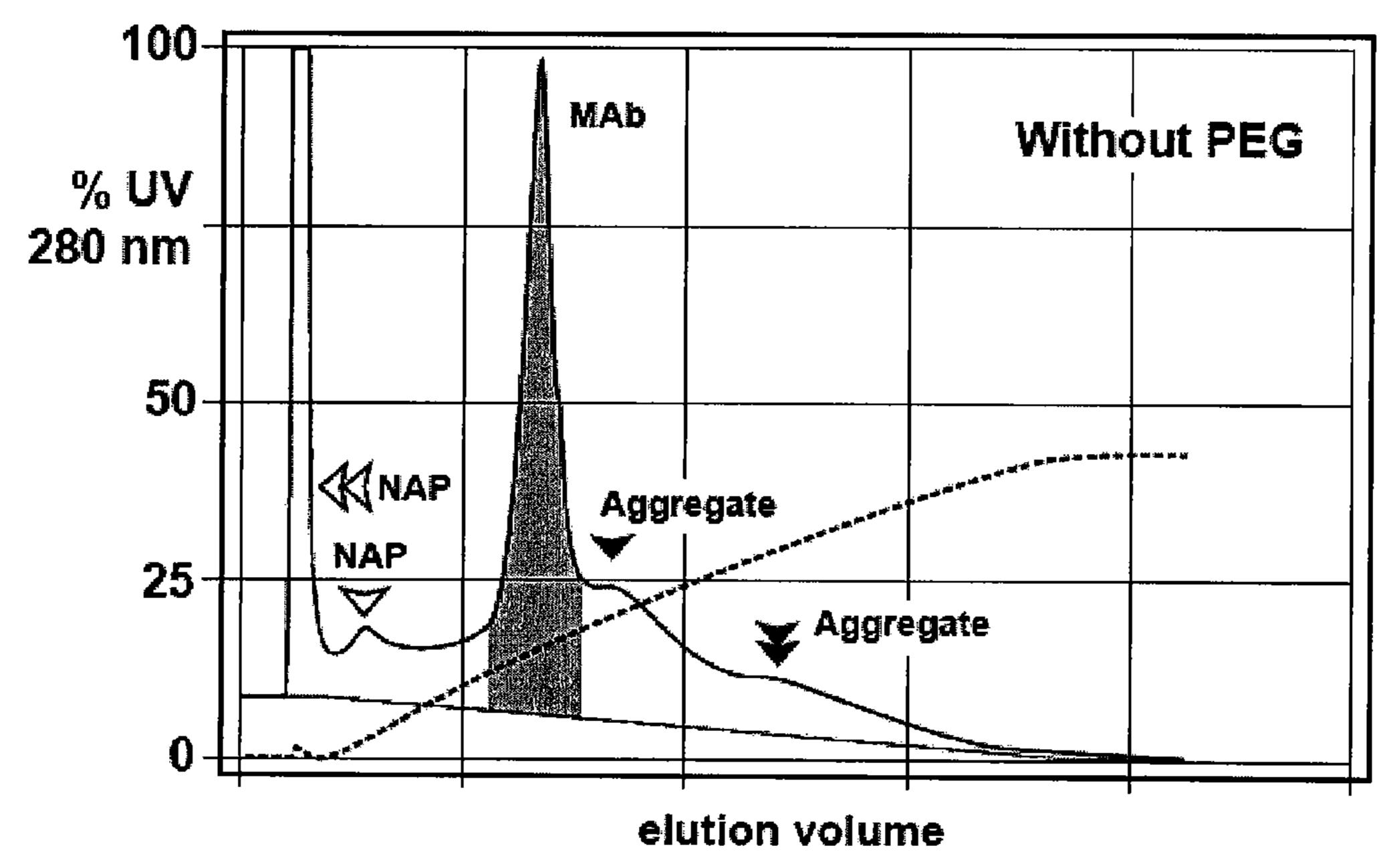
CHT Type II, 20 µm, 5 mm x 50 mm, unpurified chimeric IgG1 50 mL linear gradient elution from 5mM NaPO4, pH 6.7 to 330 mM NaPO4, pH 6.7, 300 cm/hr (1 mL/min)
