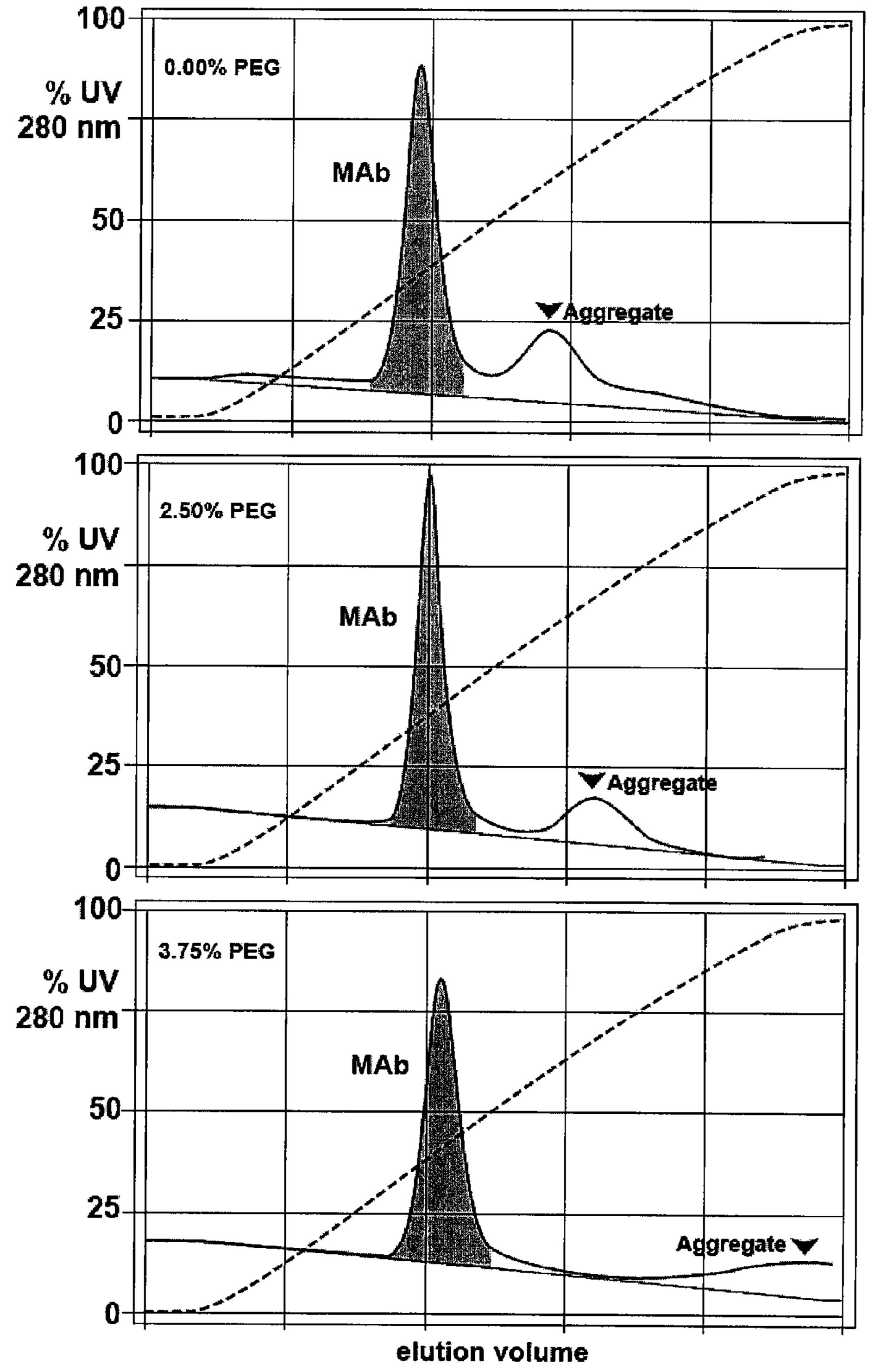
CHT Type II, 20 µm, 5 mm x 50 mm, protein A purified human IgG1 50 mL linear gradient elution from 5mM NaPO4, pH 6.7 to 5mM NaPO4, 2M NaCl, plus PEG-6000 as indicated, pH 6.7 600 cm/hr (2 mL/min)
