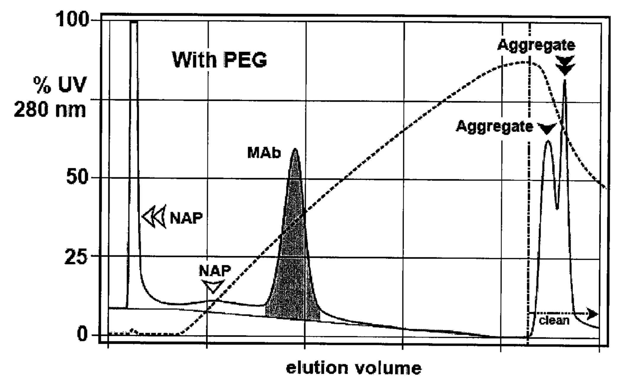
CHT Type II, 20 µm, 5 mm x 50 mm, unpurified chimeric IgG1 50 mL linear gradient elution from 5mM NaPO4, pH 6.7 to 5mM NaPO4, 2M NaCl, 5% PEG-6000, pH 6.7. Clean with 500mM NaPO4, 300 cm/hr (1 mL/min)
