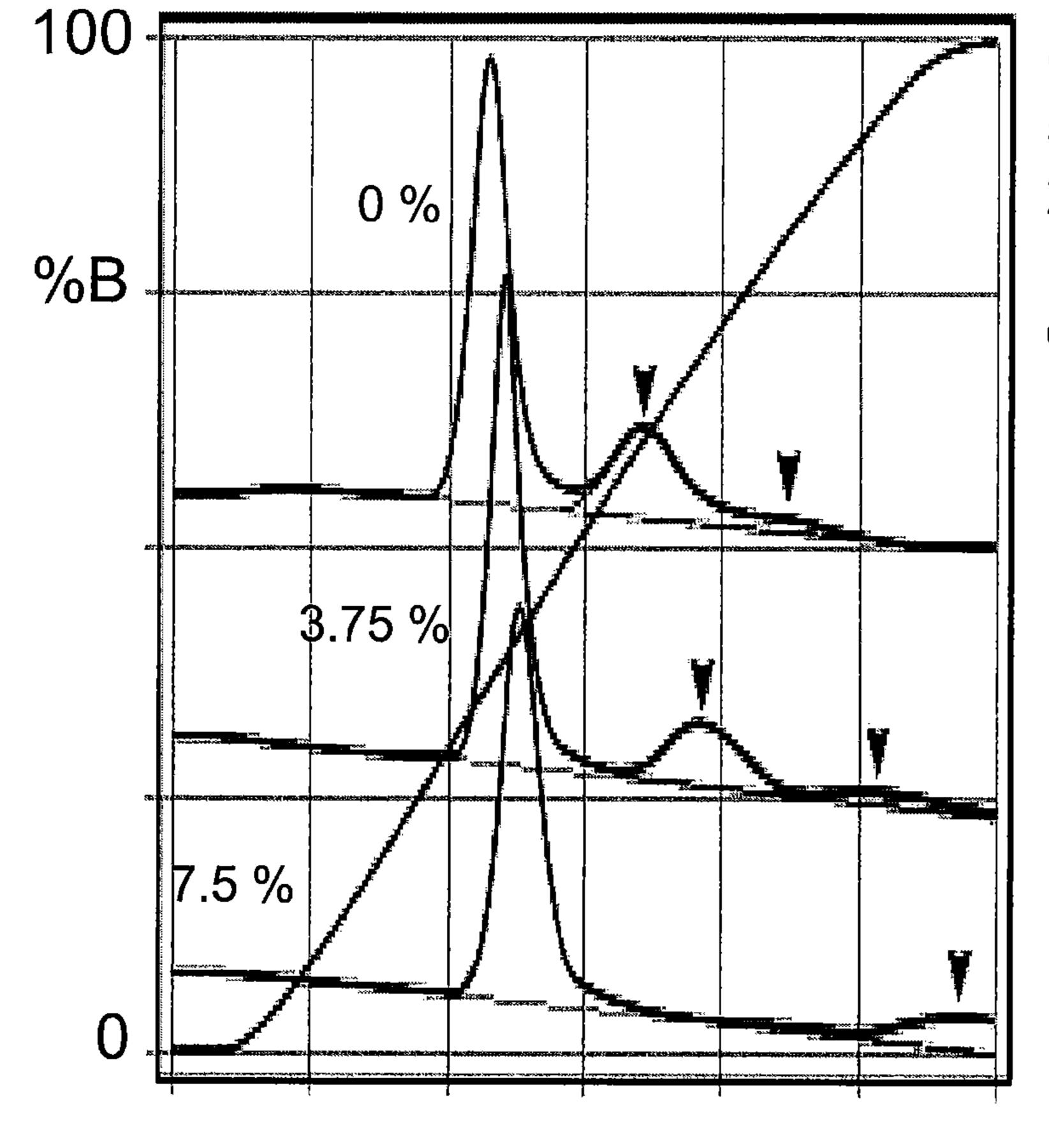
CHT I, 20  $\mu$ m 5 x 50 mm 20 CV LG, A to B 1 mL/min, 300 cm/hr chimeric IgG<sub>1</sub> (a)
