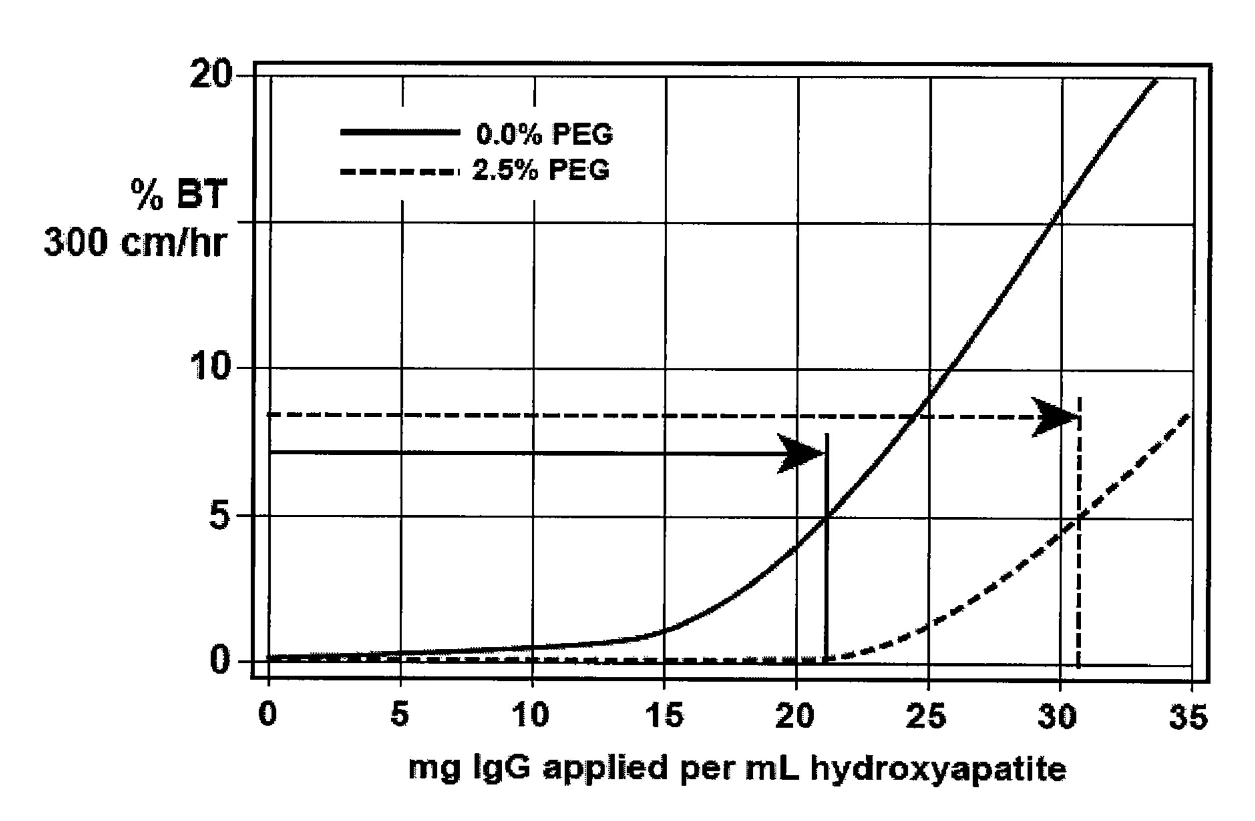
CHT Type II, 20 µm, 5 mm x 50 mm Protein A purified human IgG1, 1 mg/mL 5 mM NaPO4, pH 6.7, plus PEG-6000 as indicated
