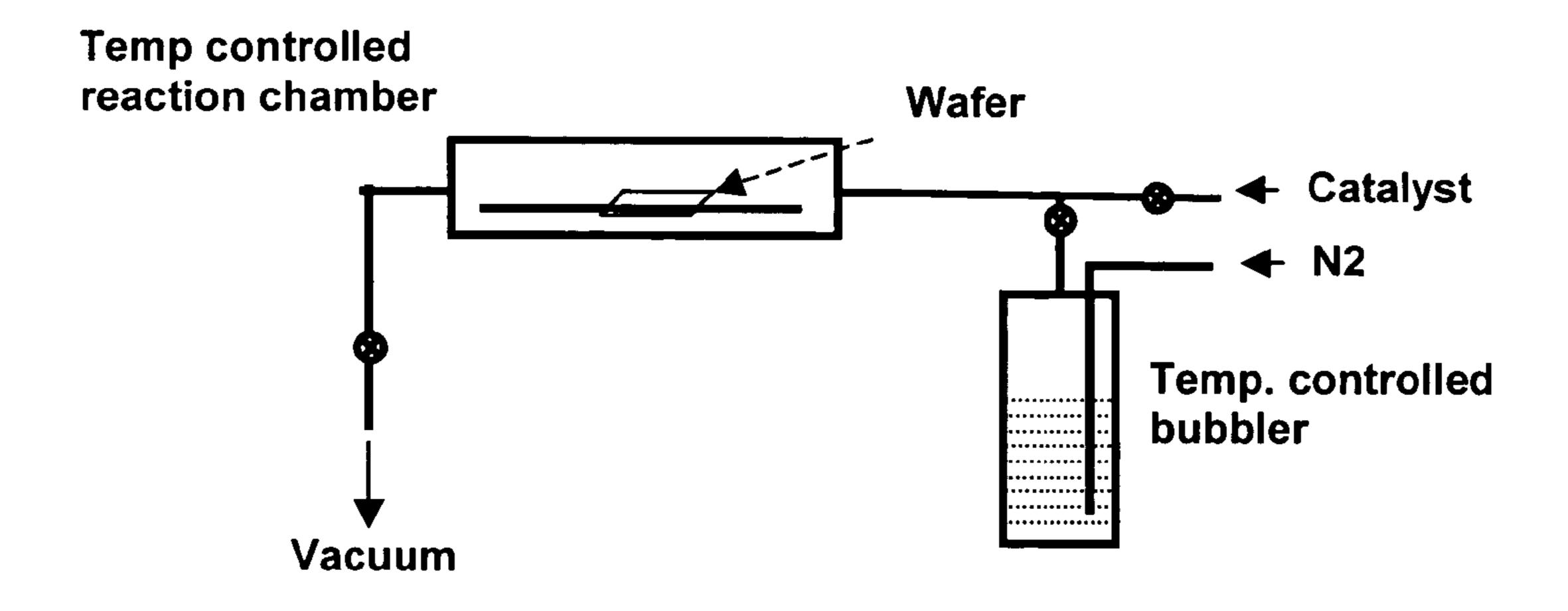
Figure 2: System Configuration B
