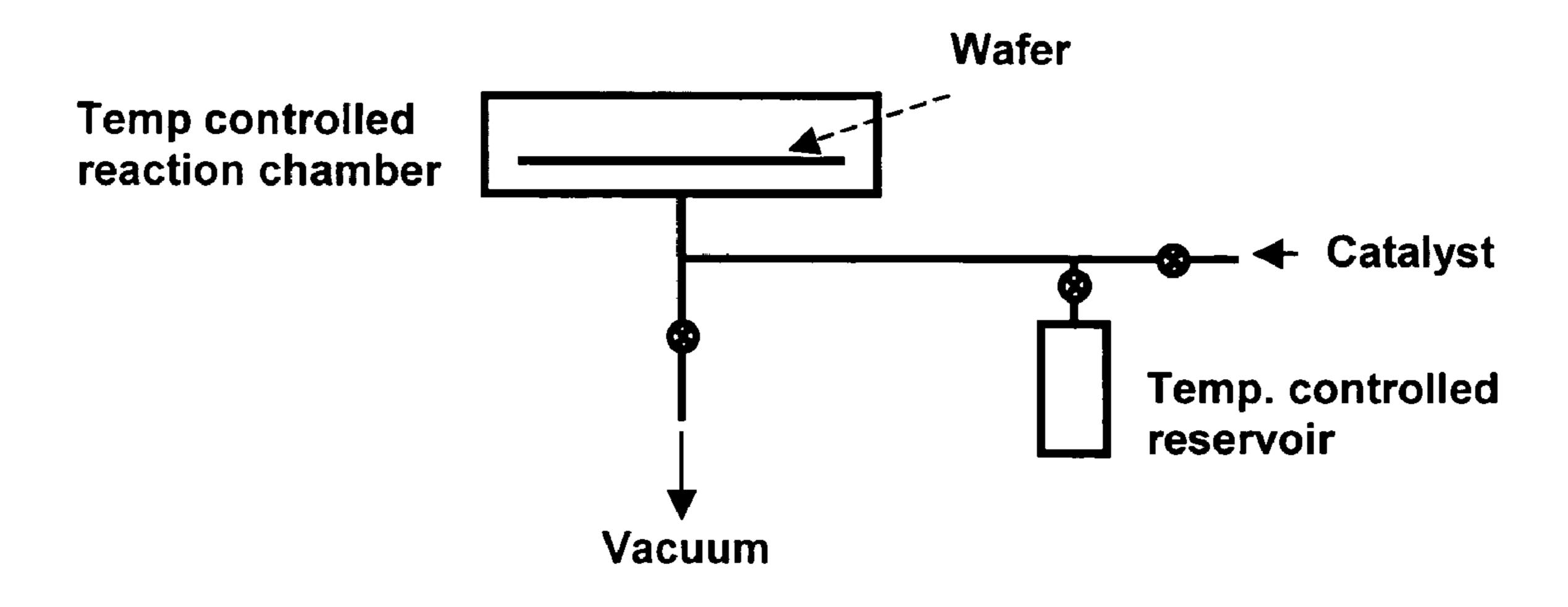
Figure 1: System Configuration A
