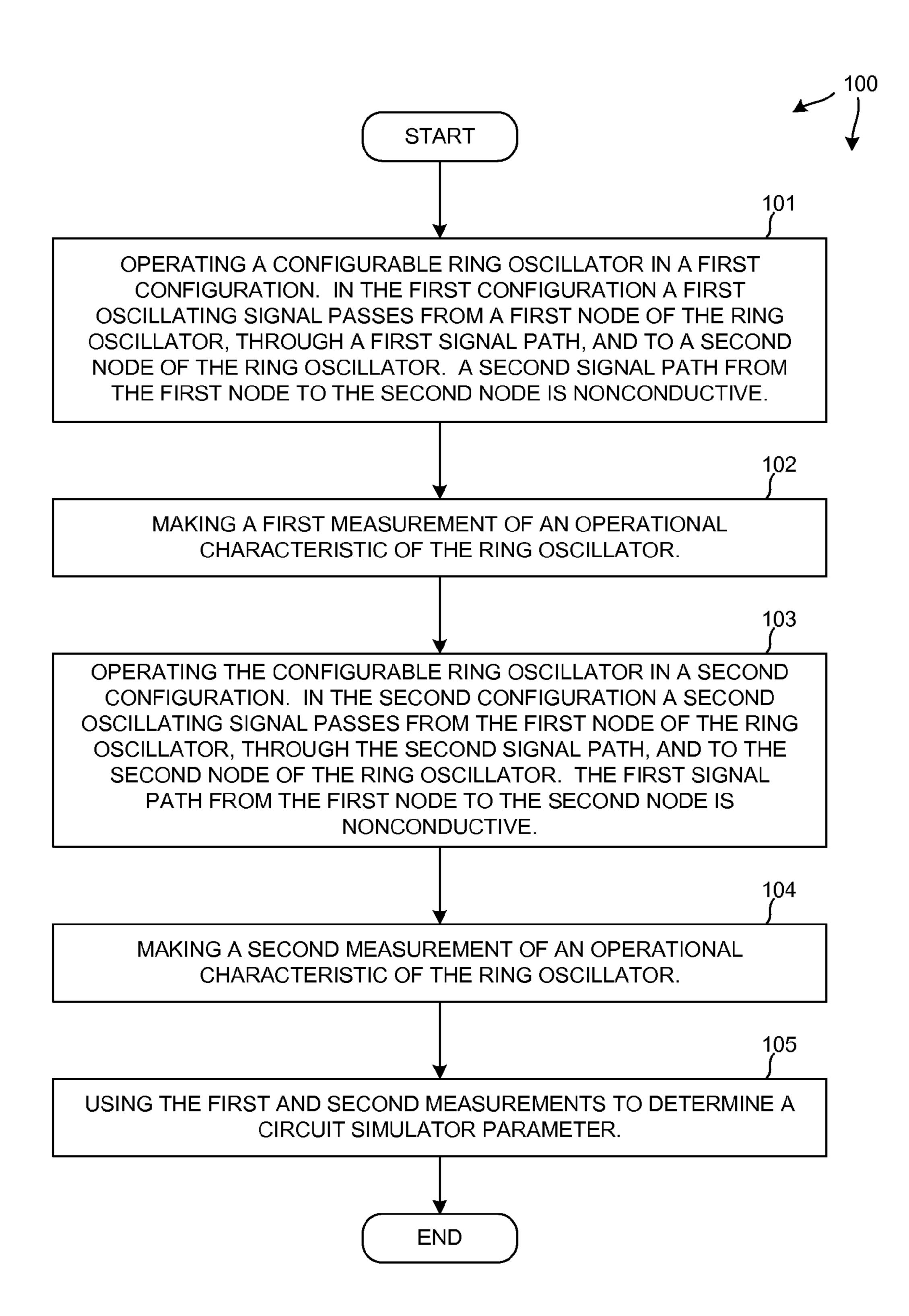
CIRCUIT SIMULATOR PARAMETER EXTRACTION METHOD
