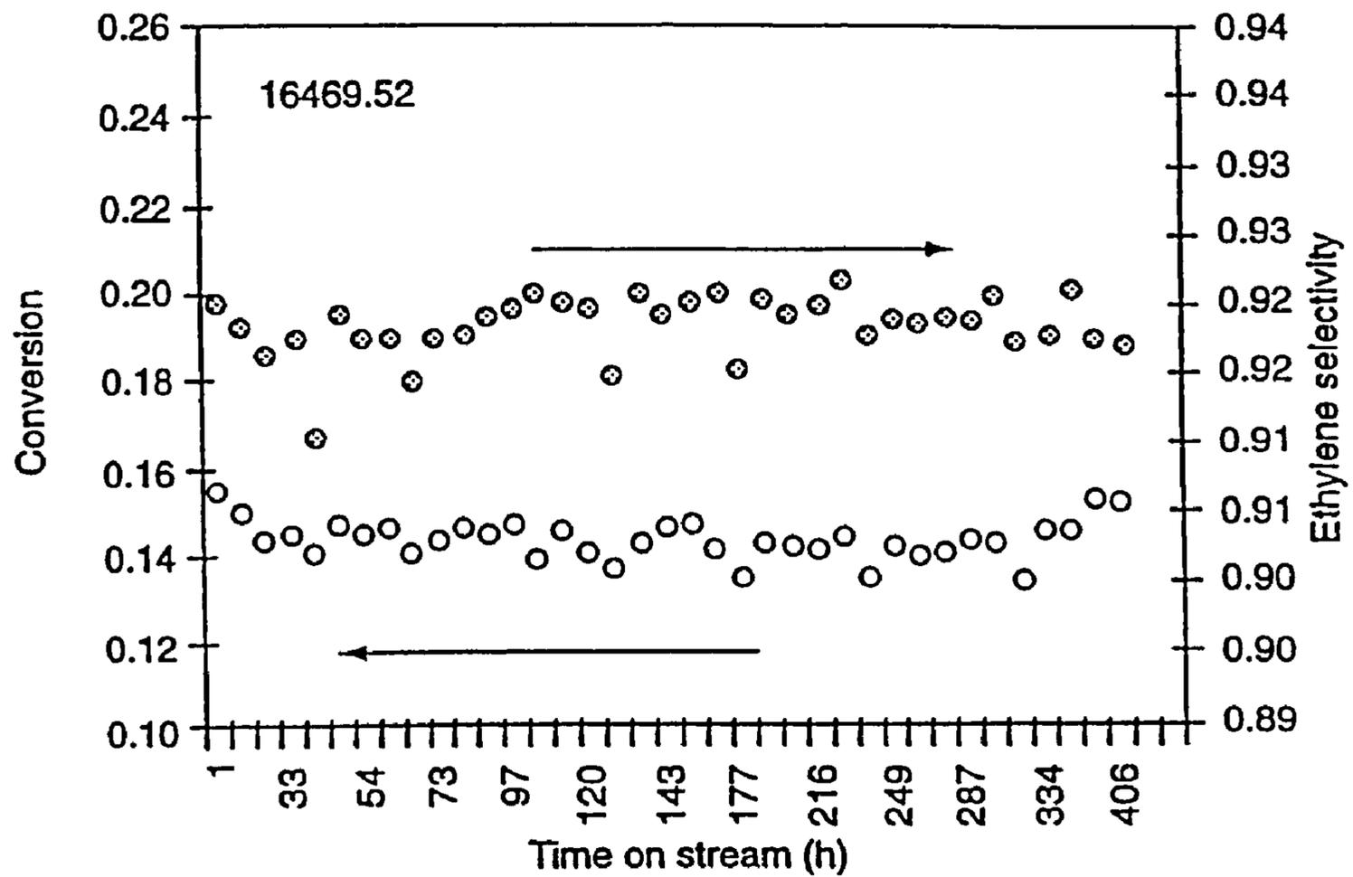
Figure 2A: Ethane conversion and ethylene selectivity over 400 hours for  $\text{Ni}_{0.75}\text{Ta}_{0.28}\text{Sn}_{0.03}\text{O}_x$  over at  $275^\circ\text{C}$
