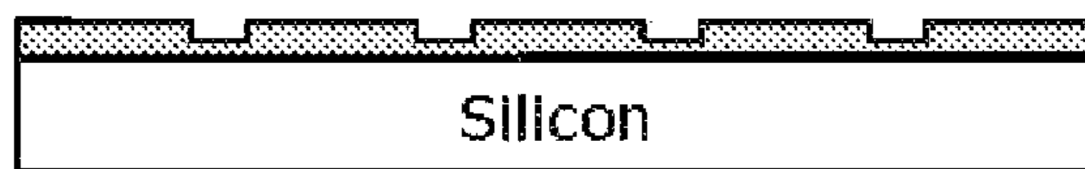
(b) LOR partial etching for bump (17 μm)
