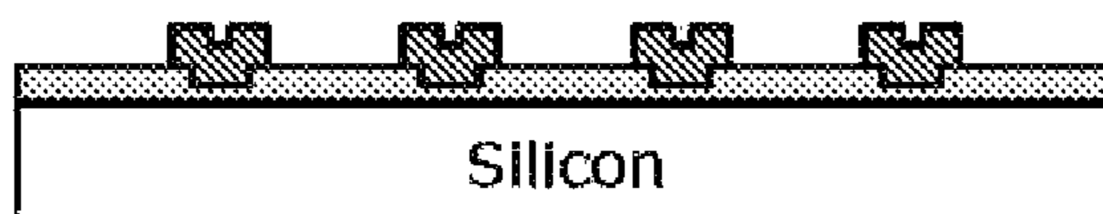
(c) Cu electroplating for metal lines (25 μm)
