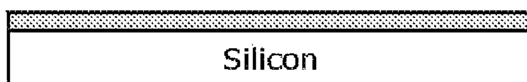
(a) Sacrificial LOR coating (24 μm)
