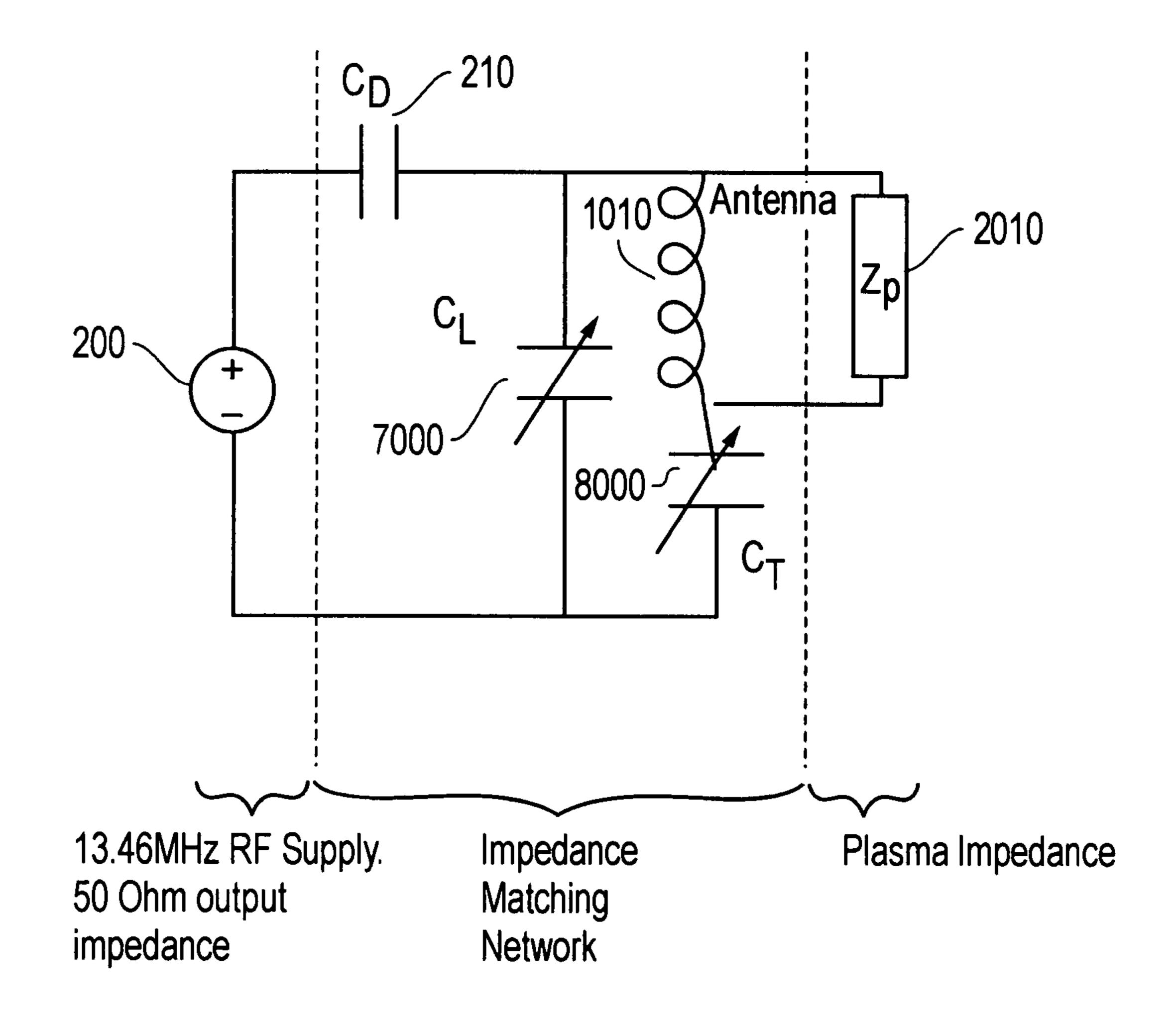
$C_D=200pF$ ,  $C_L=92pF$ ,  $C_T=216pf$ , Phase shift across antenna  $=0^\circ$ C<sub>D</sub>=50pF, C<sub>L</sub>=330pF,C<sub>T</sub>=340pf, Phase shift across antenna ≅180°
