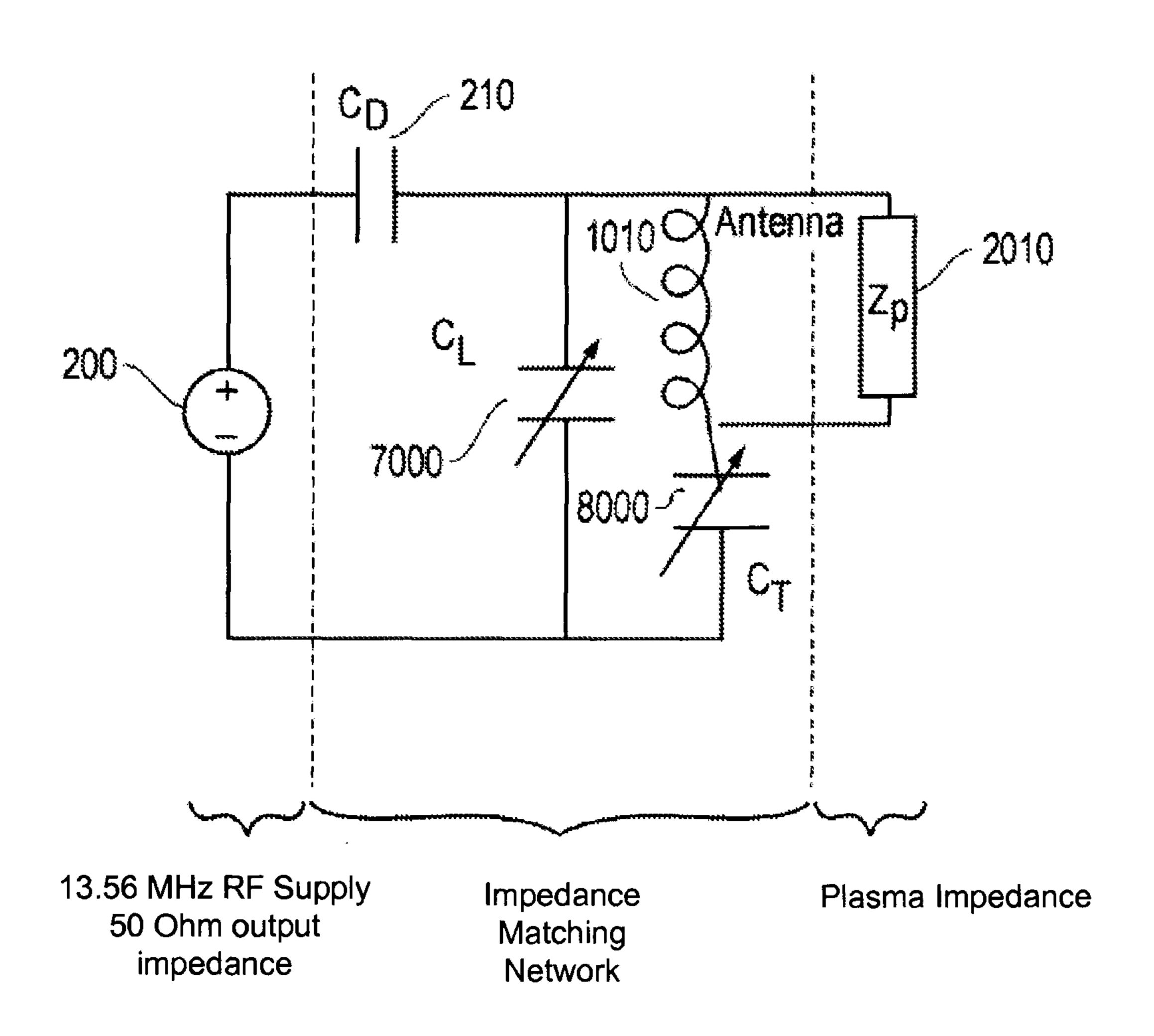
$C_D$ =200pF,  $C_L$ =92pF,  $C_T$ =216pf, Phase shift across antenna  $\cong$ 0°  $C_D$ =50pF,  $C_L$ =330pF,  $C_T$ =340pf, Phase shift across antenna  $\cong$ 180°
