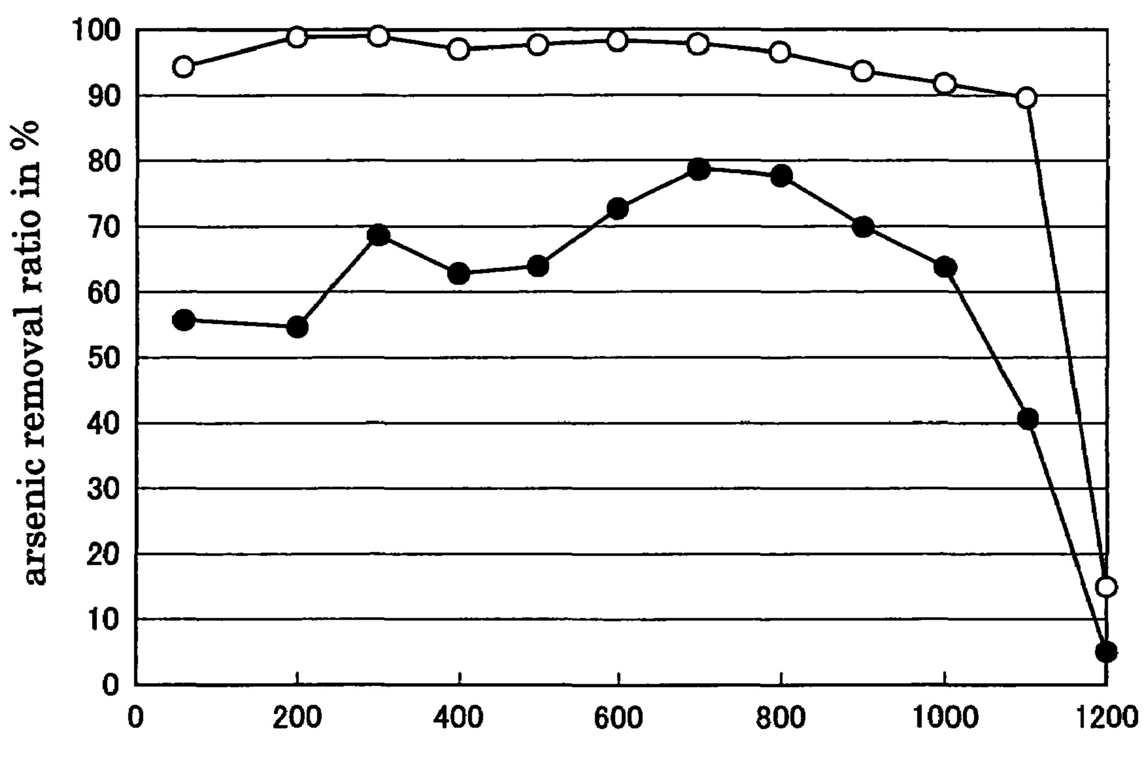
drying (baking) temperature in °C
