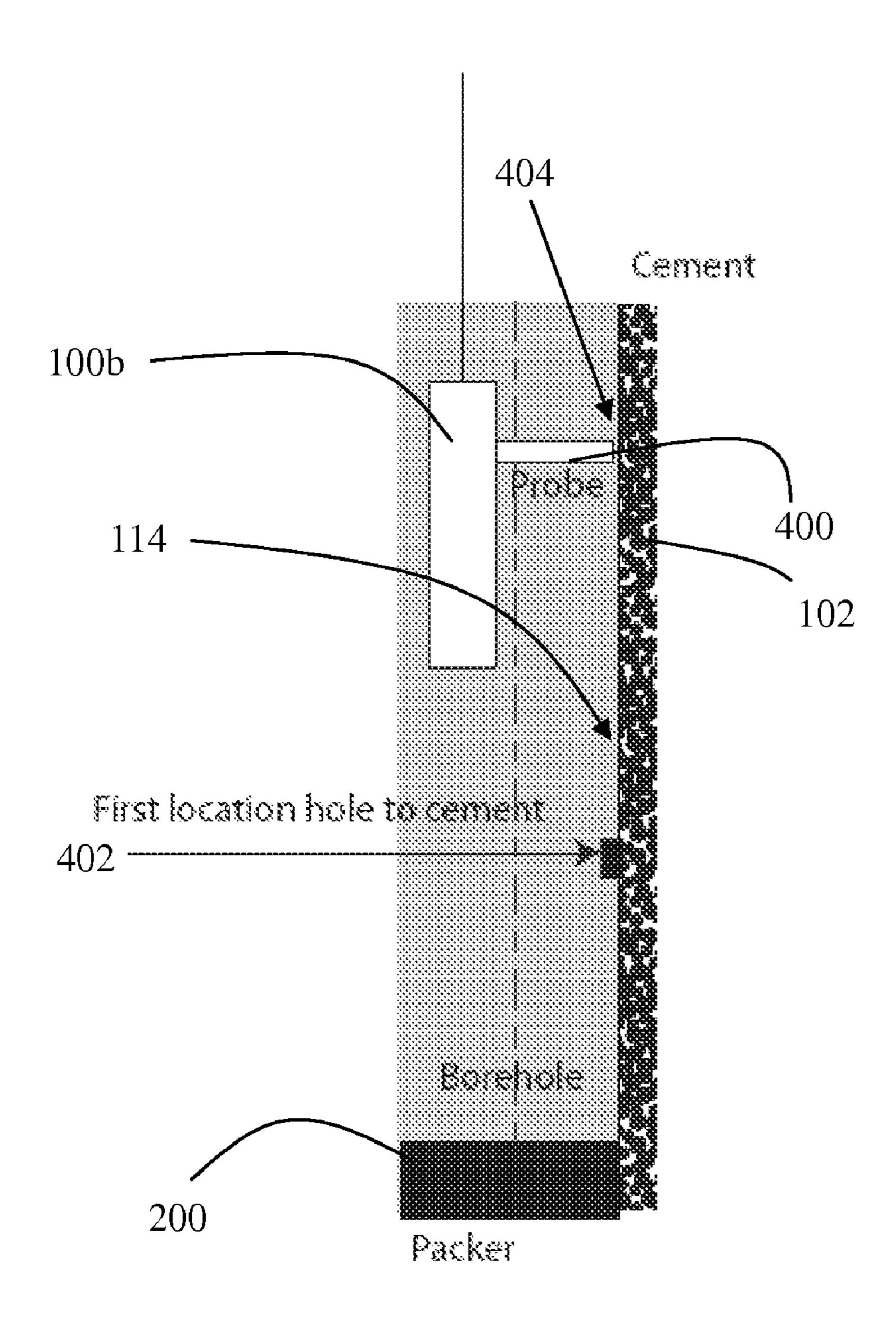
Figure 3: Illustration of the second method of cement testing.
