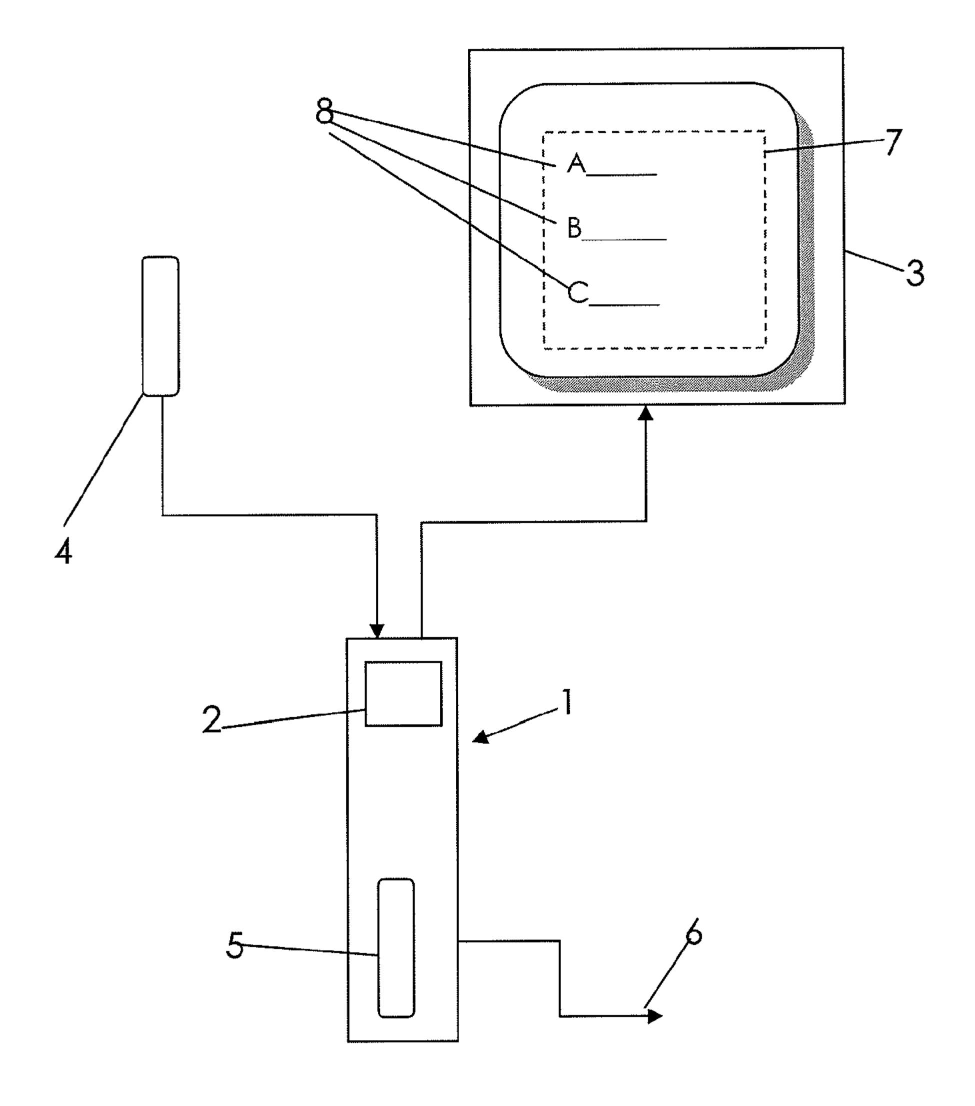
1: computing device, 2: software, 3: display unit, 4: Data intake unit, 5: Data storage unit,
