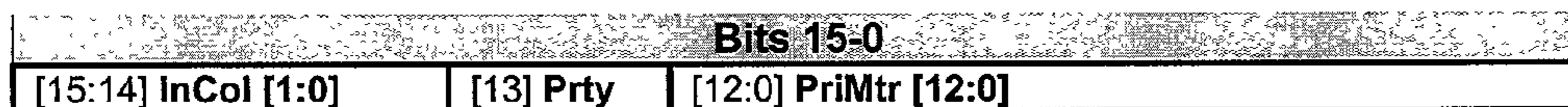
FIGURE 11 PRIMARY METER SELECTOR FORMAT
