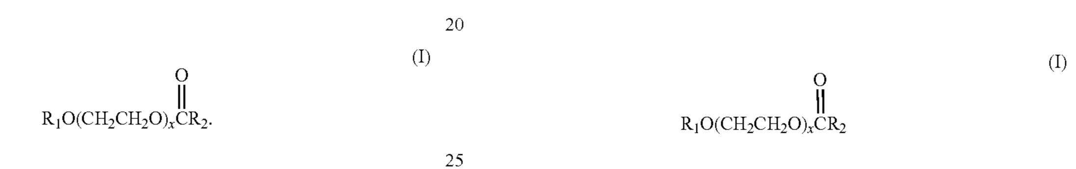
wherein  $R_1$  is a  $C_1$  hydrocarbon (methyl), linear or branched, and mixtures thereof,  $R_2$  is  $C_7$  to  $C_{22}$  hydrocarbon, linear or branched, and mixtures thereof, and the index of x is greater than or equal to 3.
