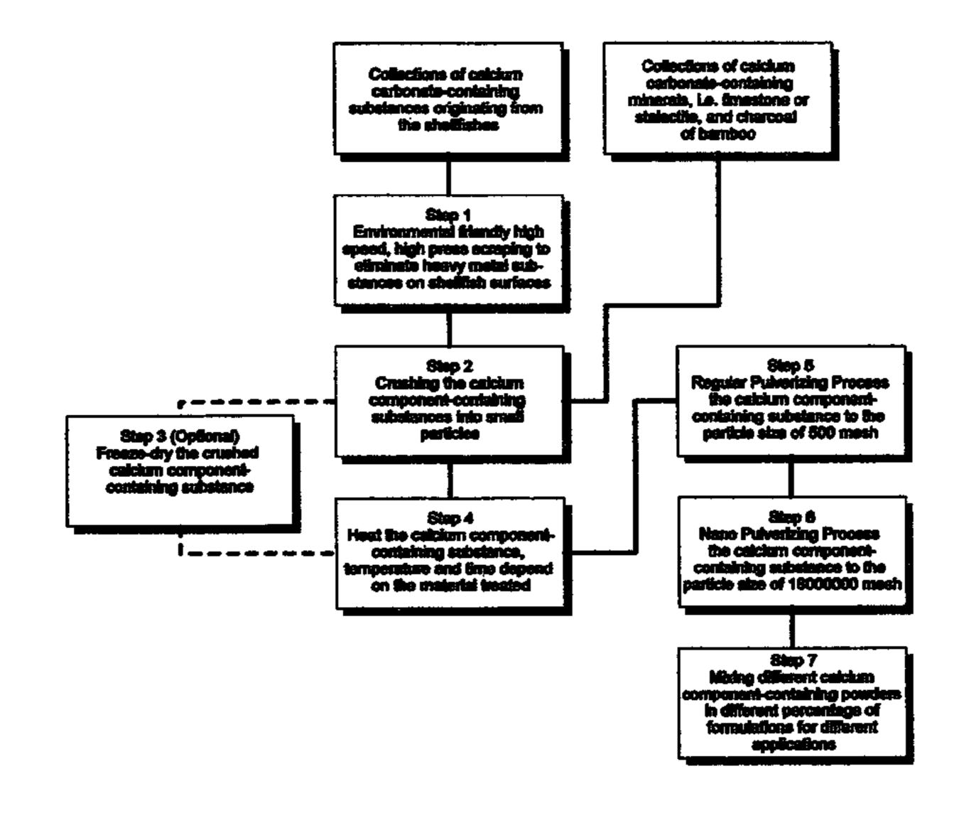
FIG. 1 - Flow chart of producing acid-neutralizing agent
