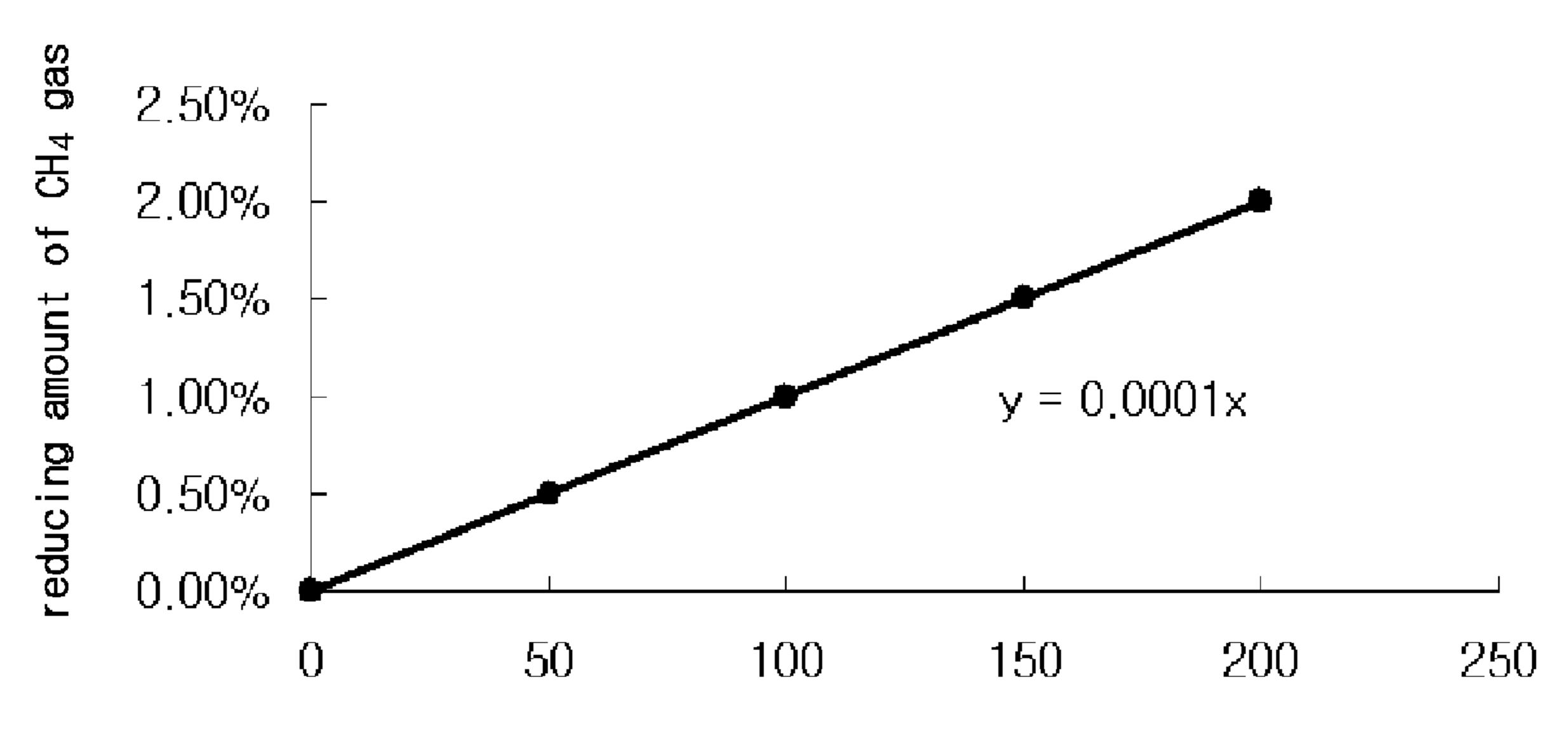
injecting amount of fine carbonaceous materials (Kg/t-p)
