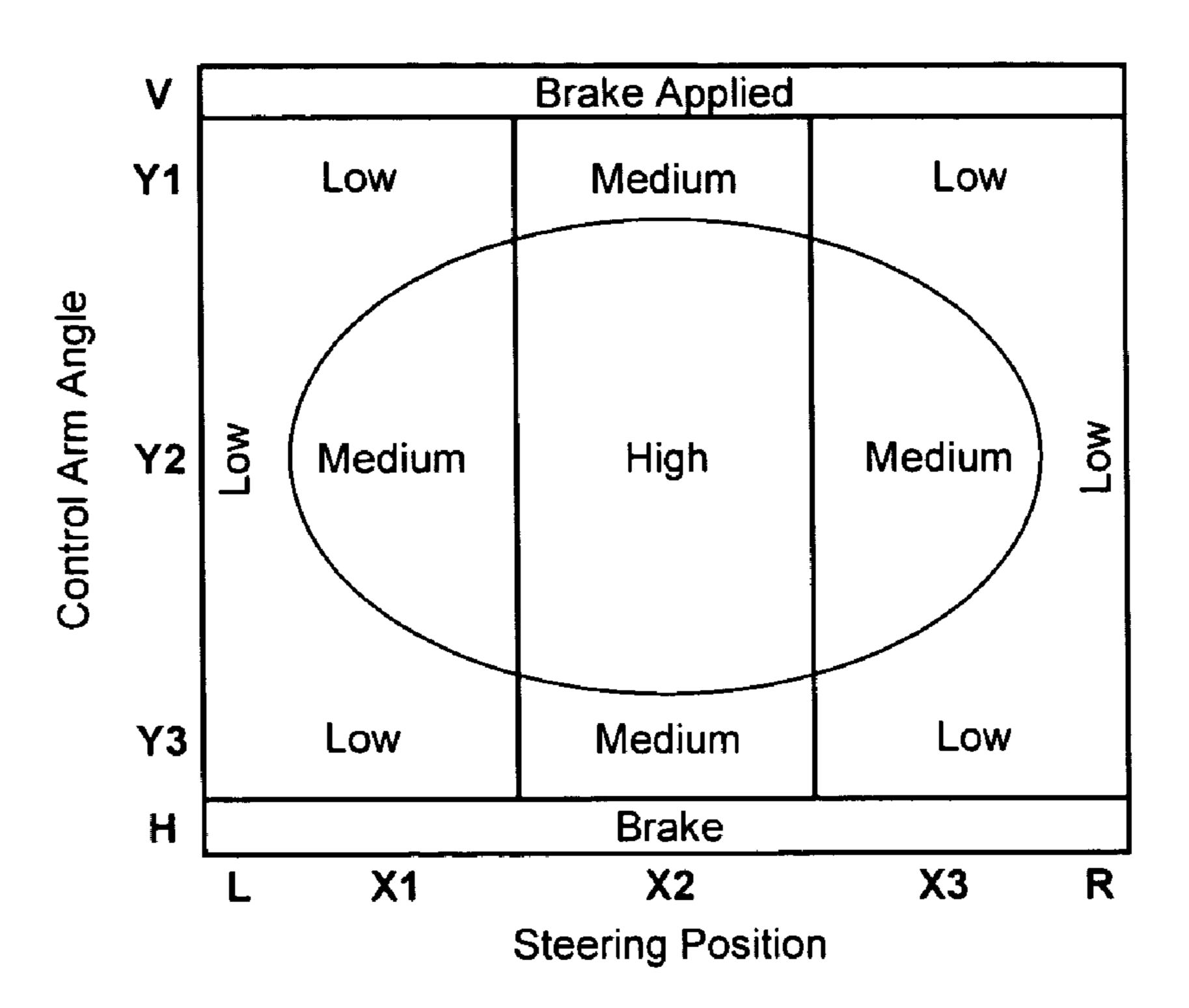
Power Assist Steering - Permissible Torque Assistance Provided by Steer Motor
