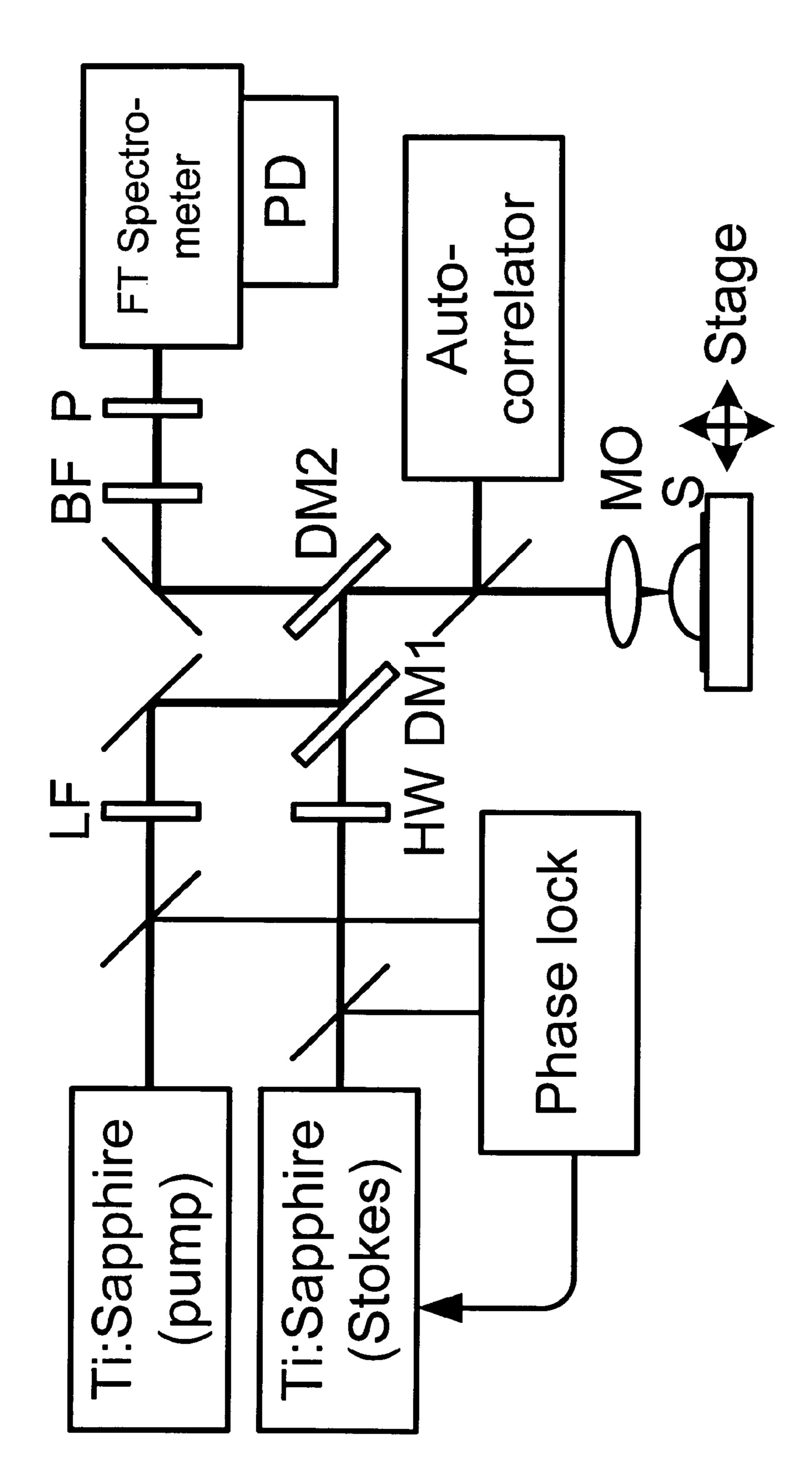
LF, laser line filter; HW, half-waveplate; DM, dichroic mirror; PD, photodiode
