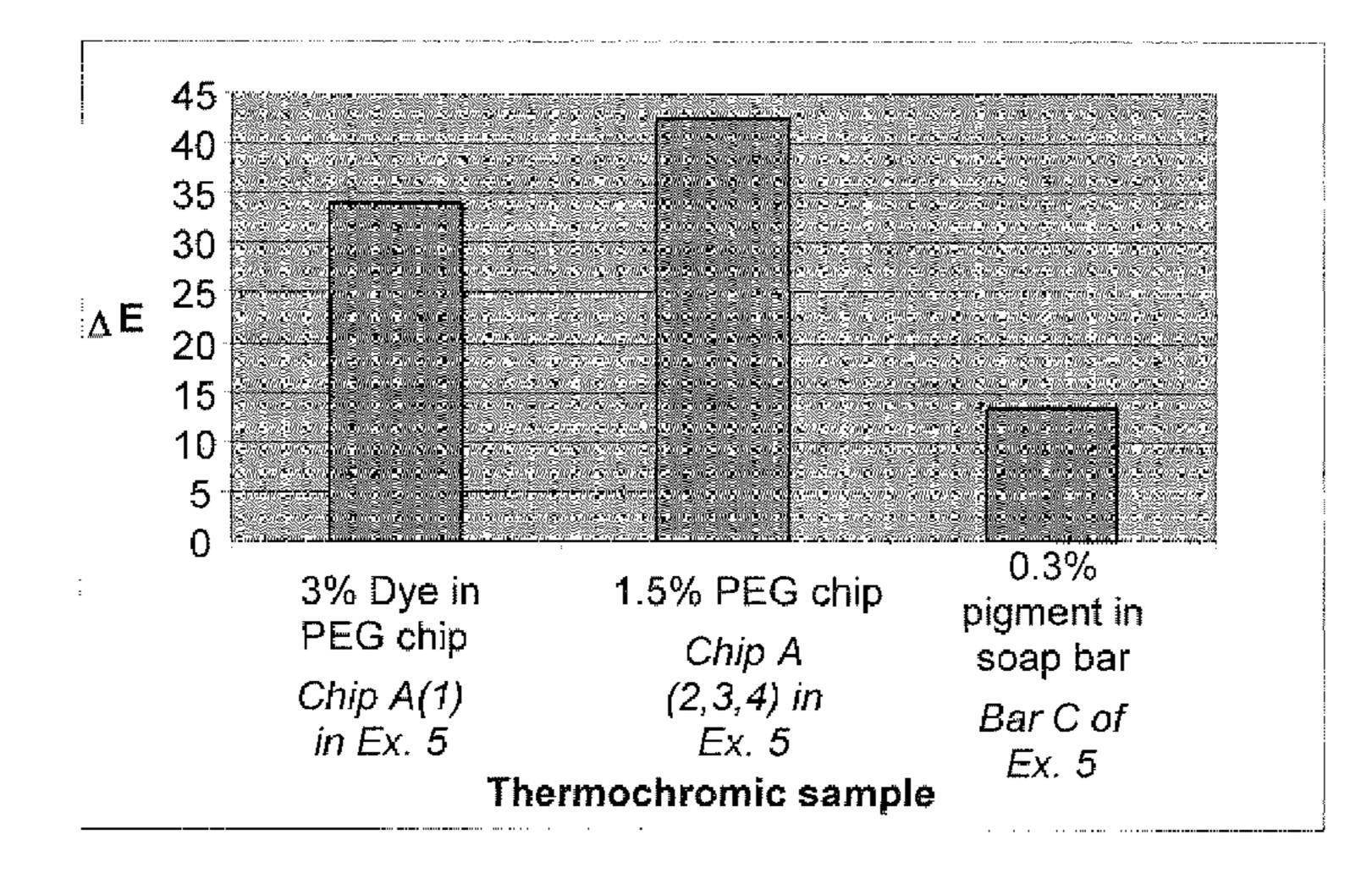
This figure shows  $\Delta E$  for PEG-8000 chip containing 3% and 1.5% thermochromic pigment (chip A(1) of Example 5 is 3% dye in chip and chips A(2) – A(4) have 1.5% dye in chip) compared to  $\Delta E$  for soap bar containing 0.3% PEG uniformly distributed throughout the bar (bar C in Example 5). For concentrated domain (chips A(1) – A(4)), only chip was measured whereas for uniform dispersal (Bar C), entire bar can be measured for  $\Delta E$  values.
