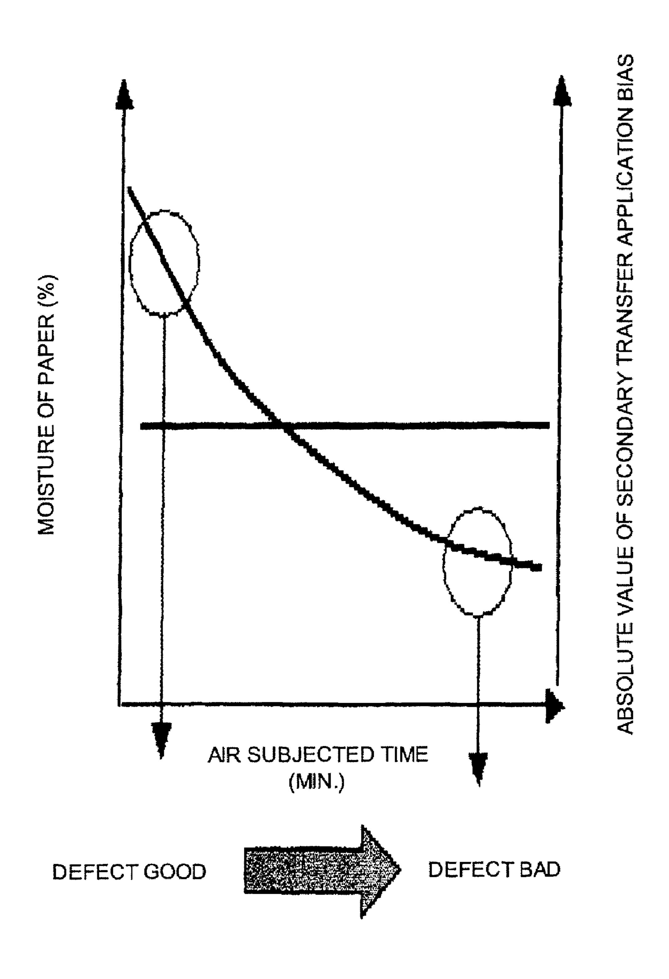
TRANSFERABILITY OF SECONDARY COLOR LOWERS THEREBY PRODUCING DEFECTED IMAGE WHEN CONTINUOUSLY APPLYING SAME TRANSFER BIAS
