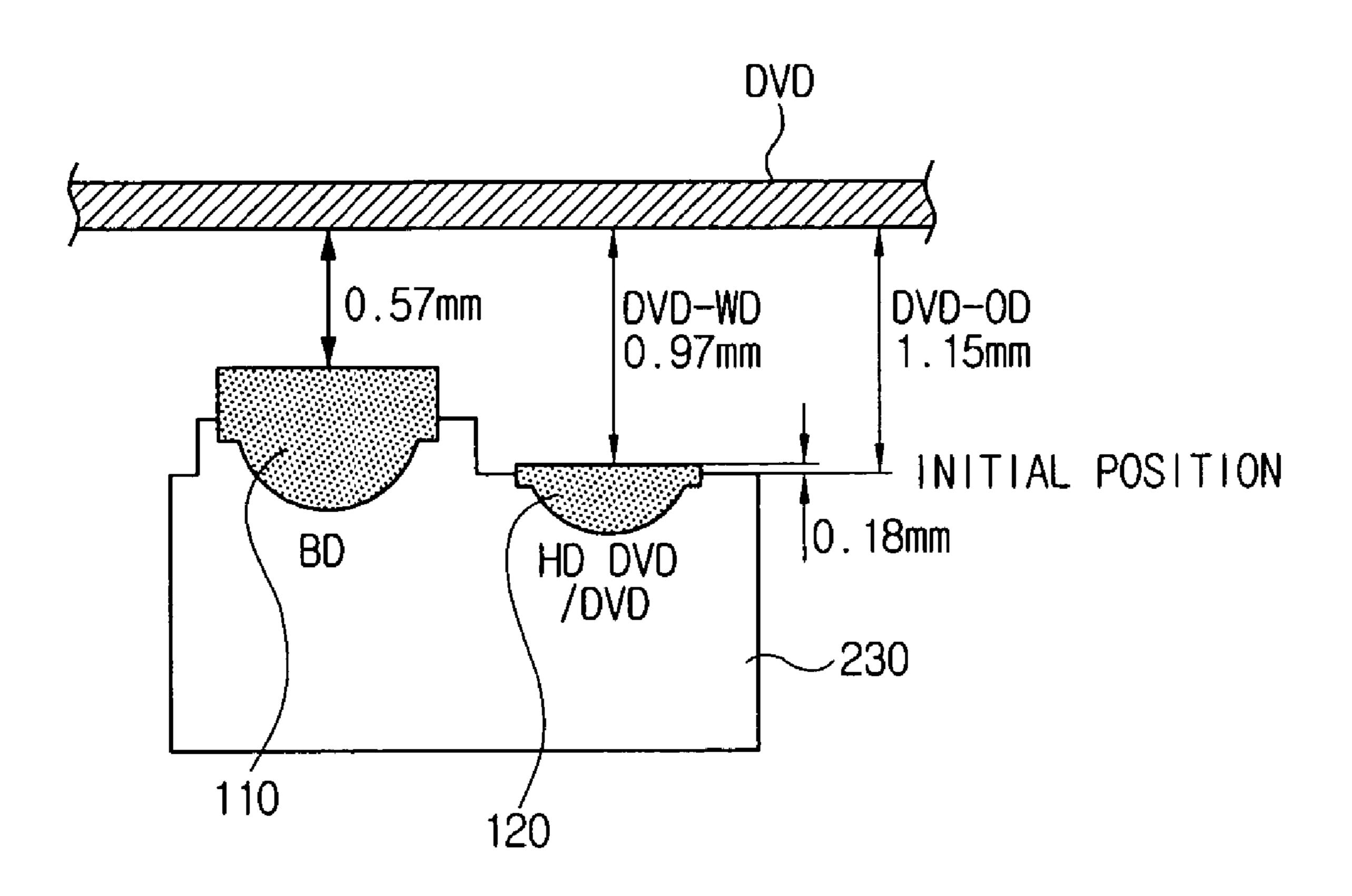
OPTICAL PICKUP FOR AN OPTICAL RECORDING AND/OR REPRODUCING APPARATUS INCLUDING AN ACTUATOR FORMING A PREDETERMINED ANGEL WITH RESPECT TO THE PICKUP BASE
