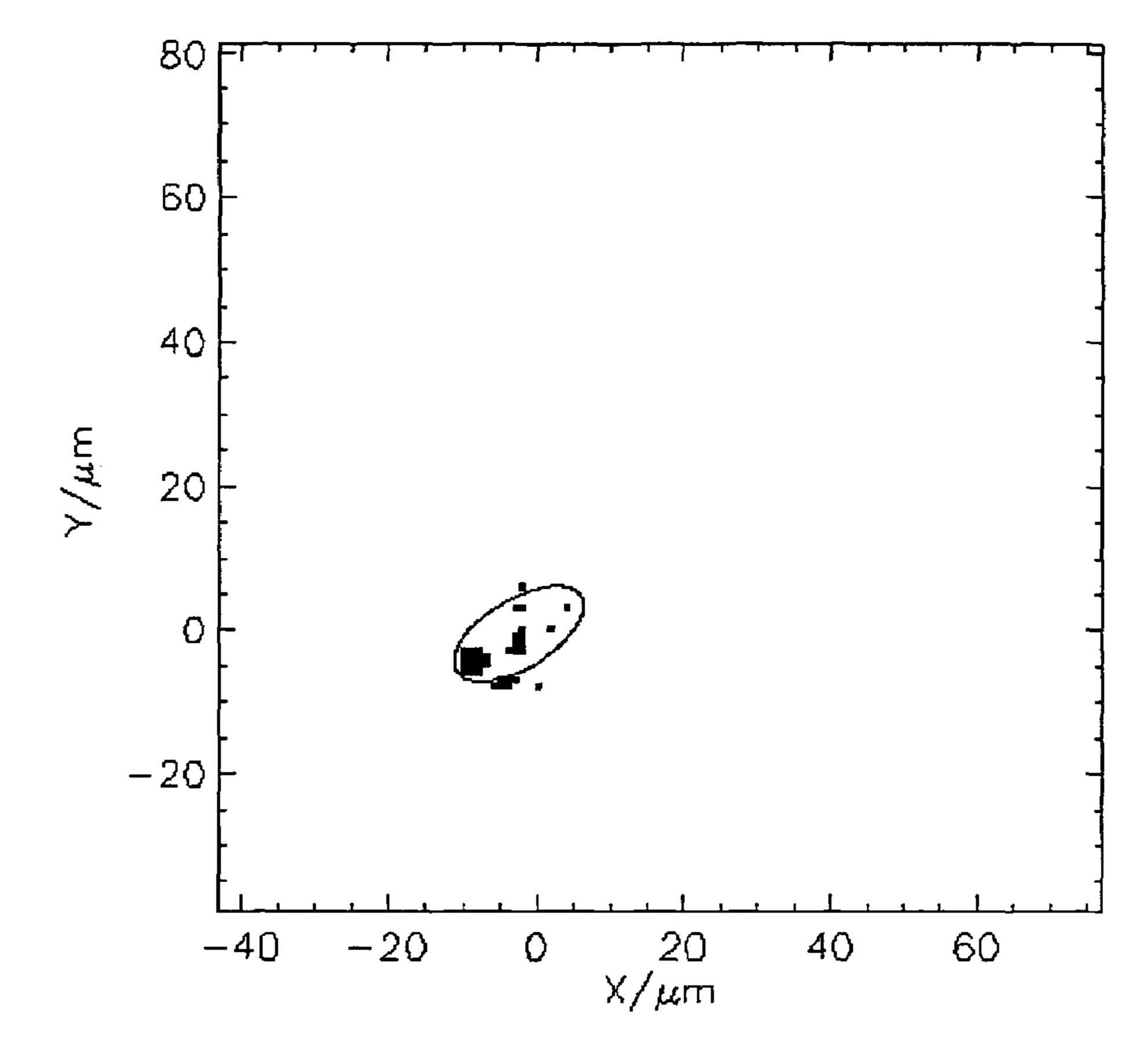
Fig.8: Parts of the PSF shown in Figure 2 which are above 50% of the maximum of intensity. The ellipse is fitted by using the area of convex hull and circle shown in Figure 7 are used for determination of the short and long axis of the ellipse.
