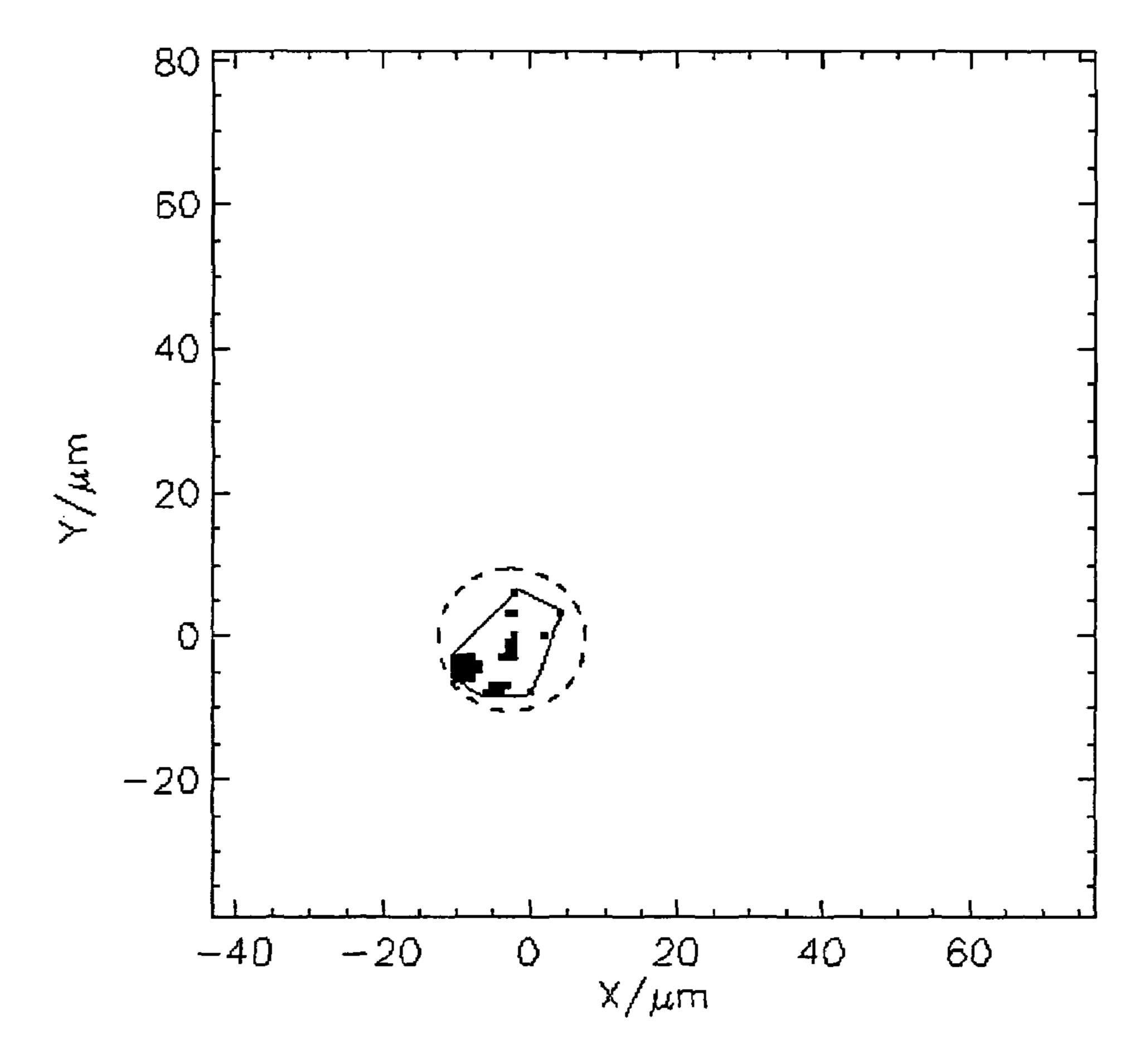
Fig.7: Parts of the PSF shown in Figure 2 which are above 50% of the maximum of intensity. The convex hull is shown by the solid line. The dashed circle circumscribes the relevant parts.
