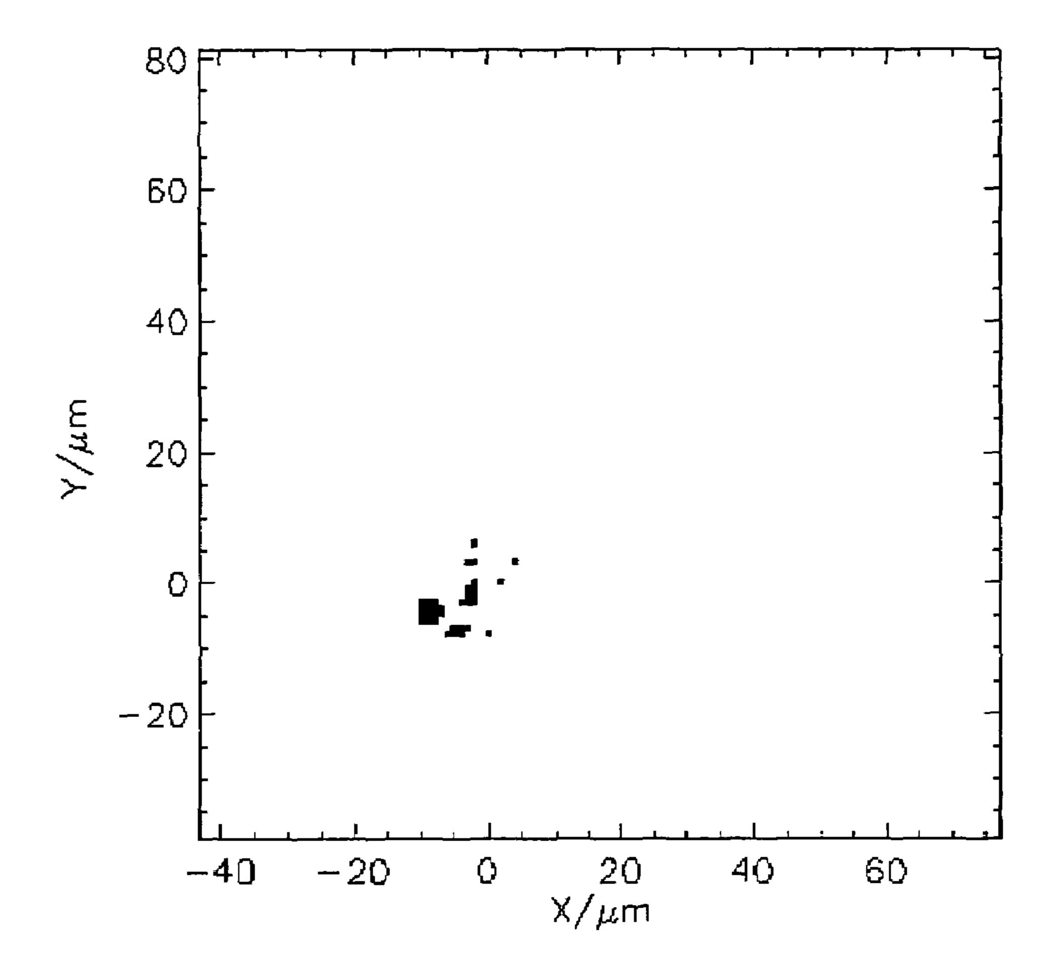
Fig.3: Parts of the PSF shown in Figure 2 which are above 50% of the maximum of intensity
