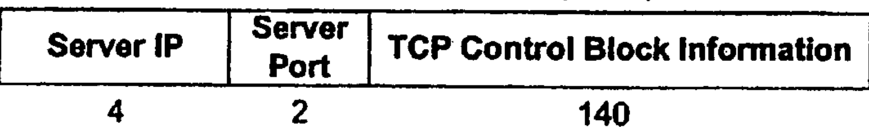
ipOS TCP Connection Packet (Type=0x01; Protocol=0x01)
