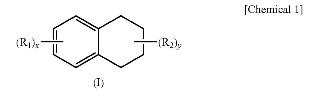
wherein x is an integer of 0 to 4; y is an integer of 0 to 8;  $R_1$  and  $R_2$  each independently represent an alkyl or alkoxy group having 1 to 10 carbon atoms or an alkenyl or alkenyloxy group having 2 to 10 carbon atoms; these groups may be substituted by a halogen atom; and when a plurality of  $R_1$  or  $R_2$  exists,  $R_1$  and  $R_2$  each may be the same or different,
