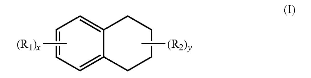
wherein x is an integer of 0 to 4; y is an integer of 0 to 8;  $R_1$  and  $R_2$  each independently represent an alkyl or alkoxy group having 1 to 10 carbon atoms or an alkenyl or alkenyloxy group having 2 to 10 carbon atoms; these groups may be substituted by a halogen atom; and when a plurality of  $R_1$  or  $R_2$  exists,  $R_1$  and  $R_2$  each may be the same or different,
