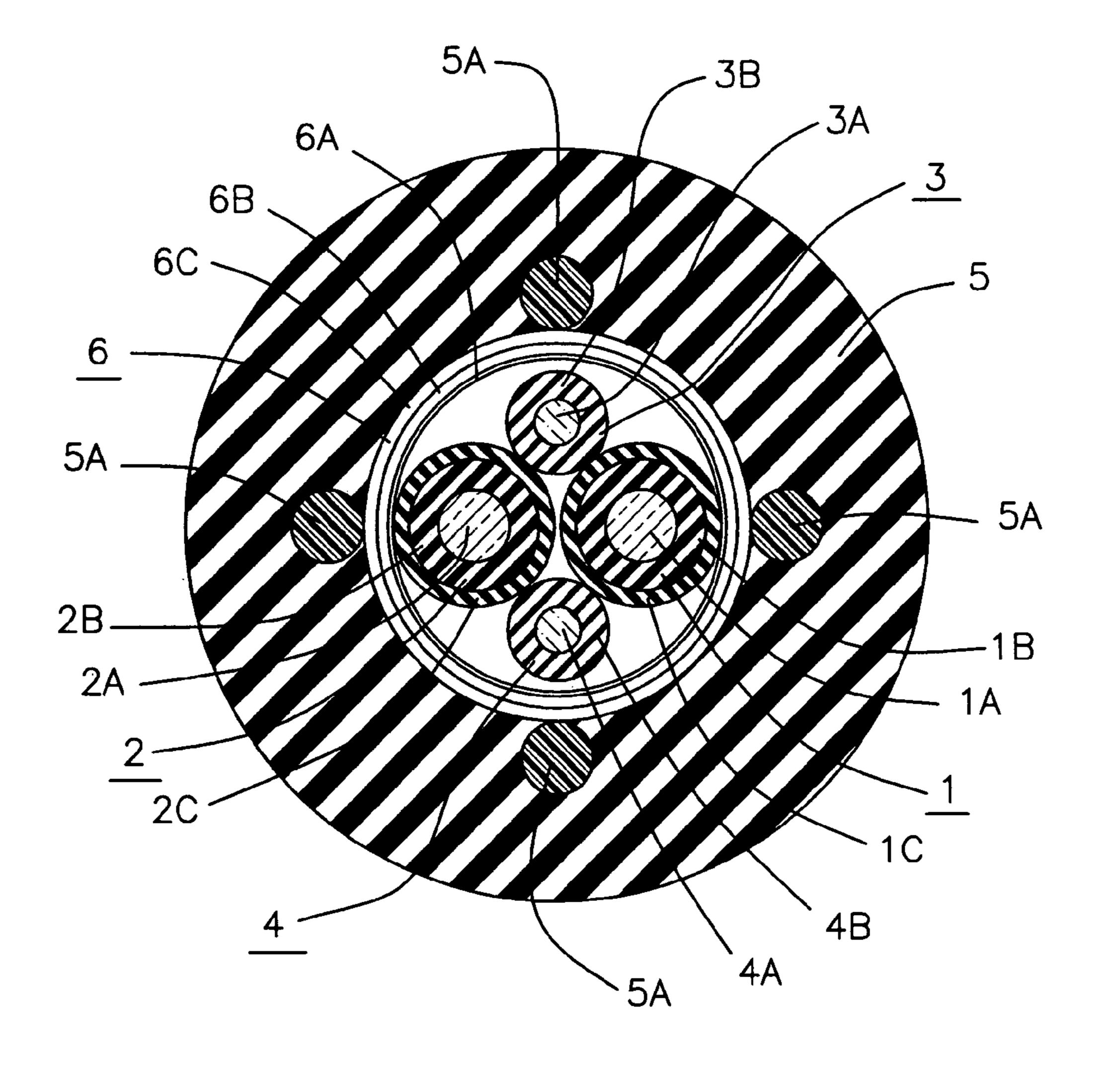
The invention relates to a composite cable to be laid by being drawn or blown into a cable tube.
