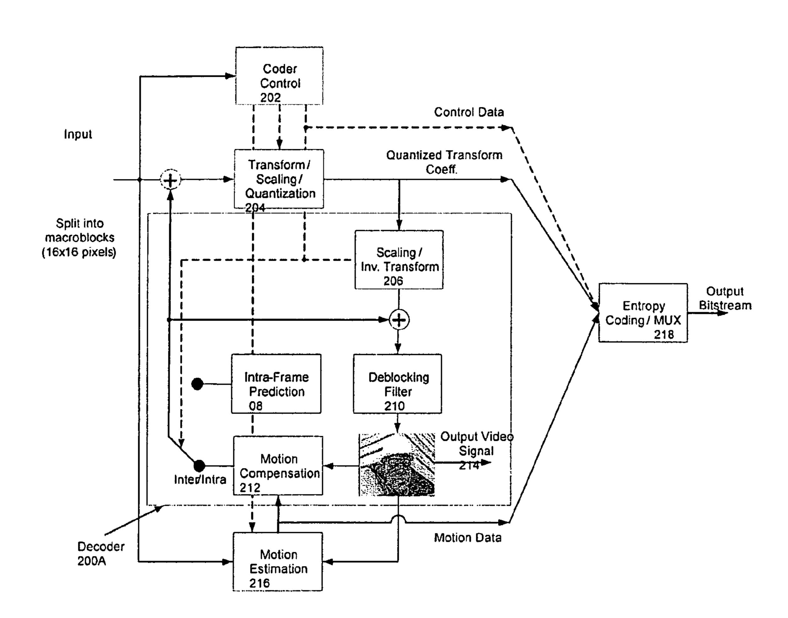
FIG. 3: Single-Layer Video Decoder
