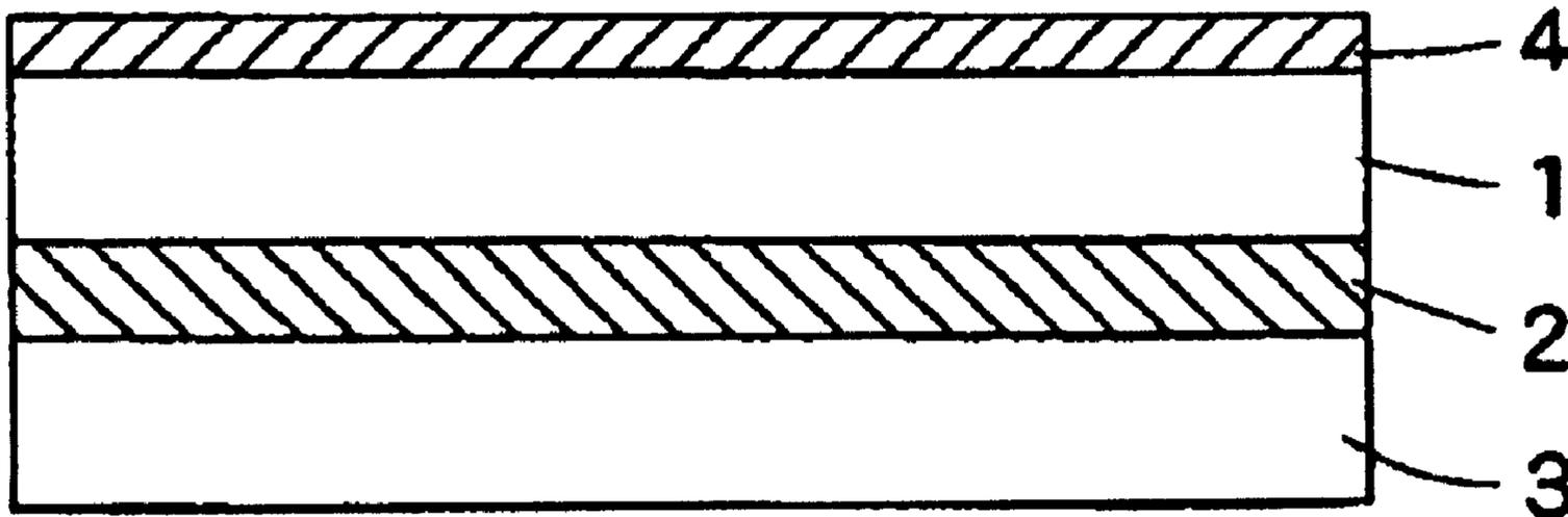
1. A thermal transfer sheet comprising: a substrate; a heat resistant slip layer; an adhesive layer; and a dye layer, wherein
