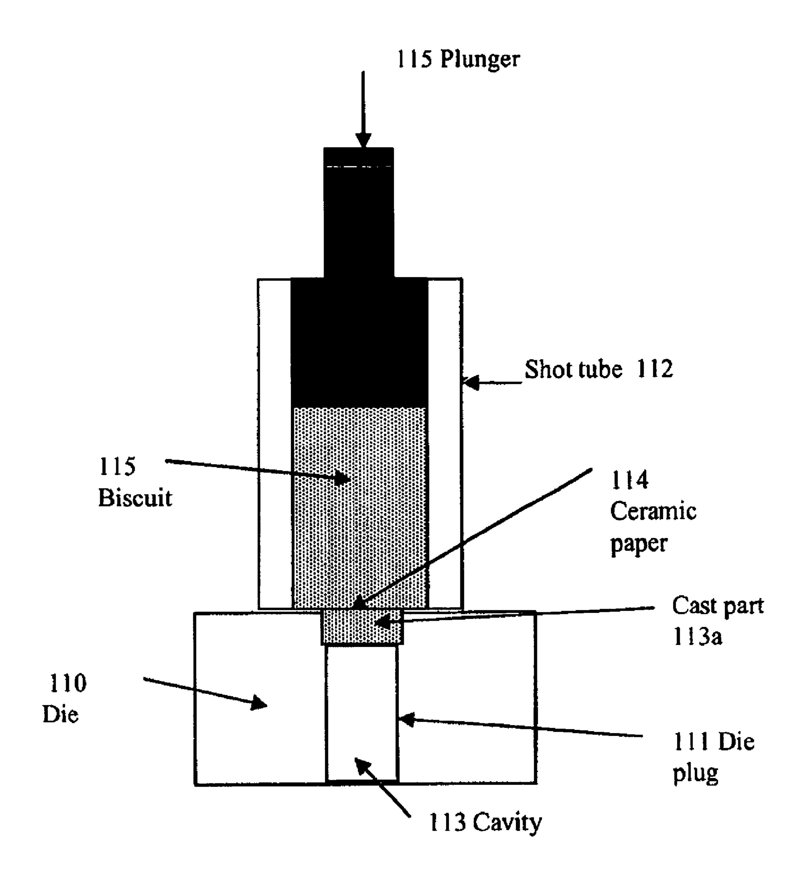
Figure 2- Schematic of the squeeze casting assembly
