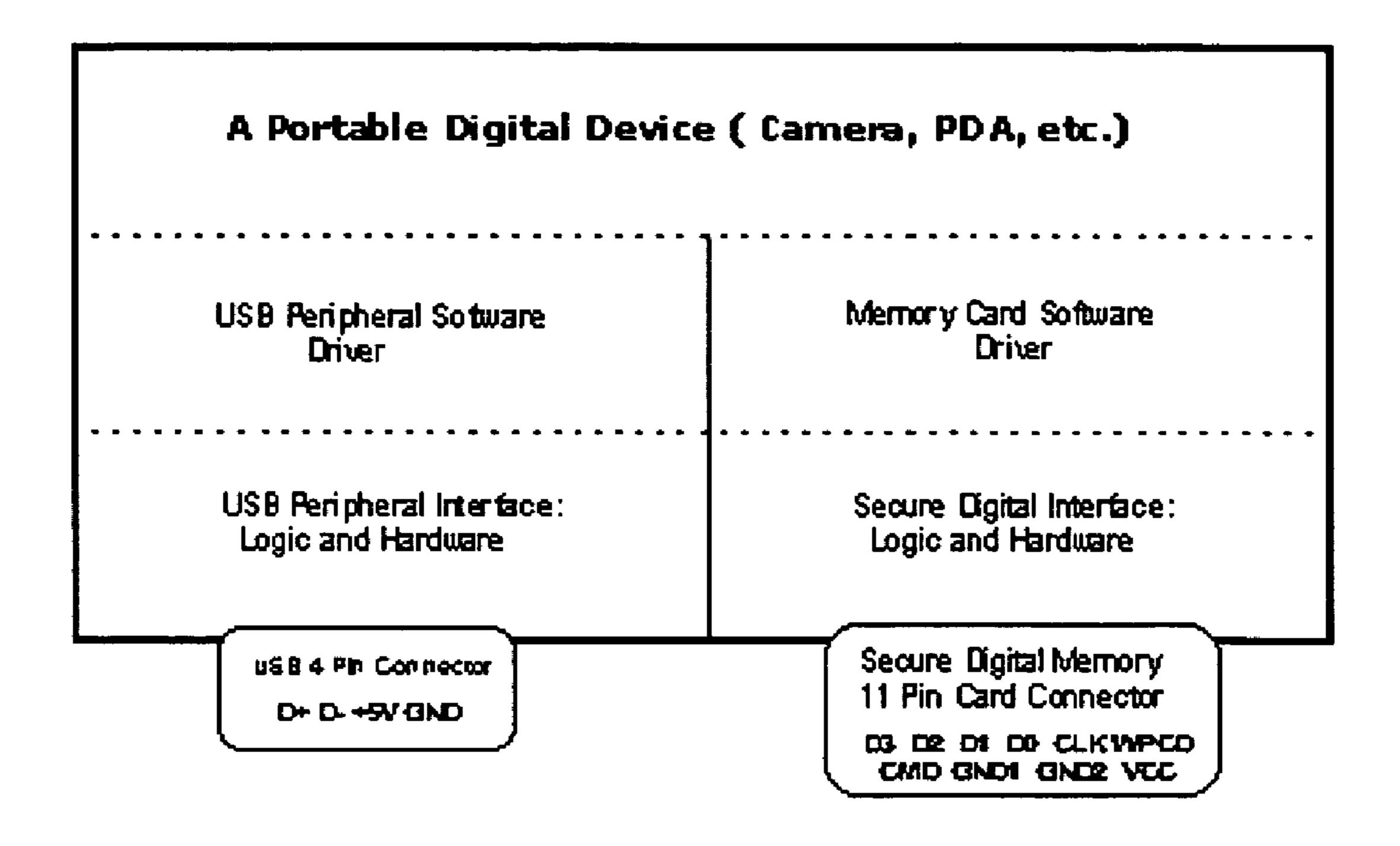
Figure 1: Interface Ports of a Typical Portable Digital Device (PDD)
