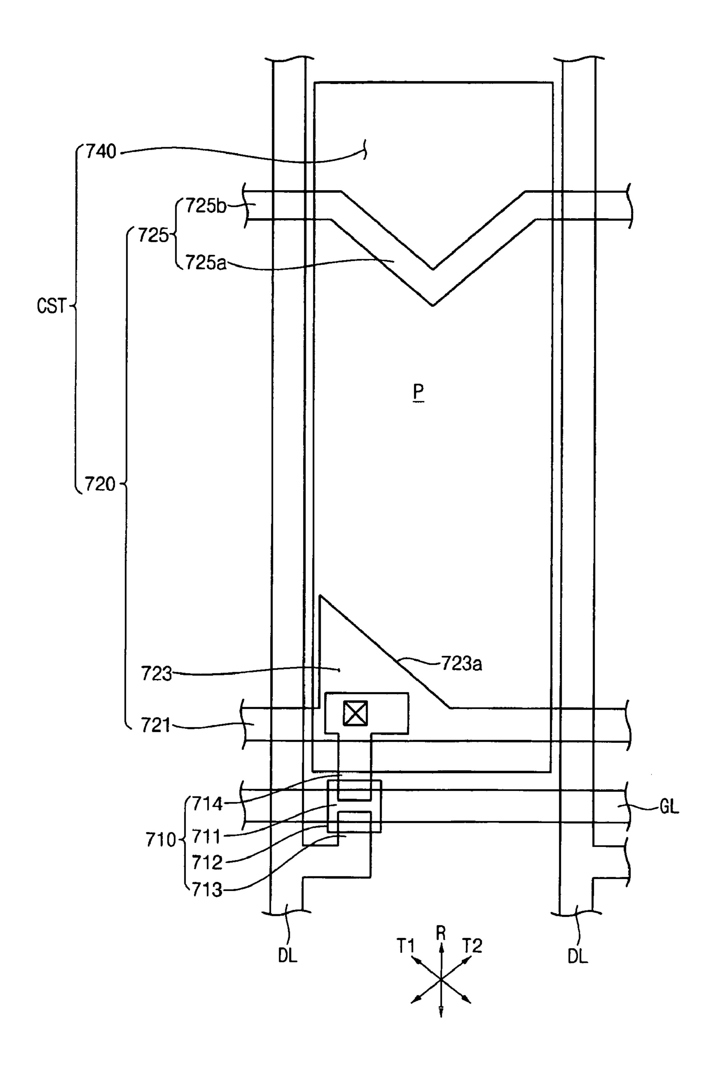
ARRAY SUBSTRATE WITH SWITCHING DEVICE AND STORAGE ELECTRODE PART FORMED OF A COMMON LINE AND BLOCKING COMMON ELECTRODE ON THE SAME PLANE AND HAVING AN OBLIQUE SIDE PARALLEL WITH TRANSMISSION AXIS OF POLARIZING PLATE
