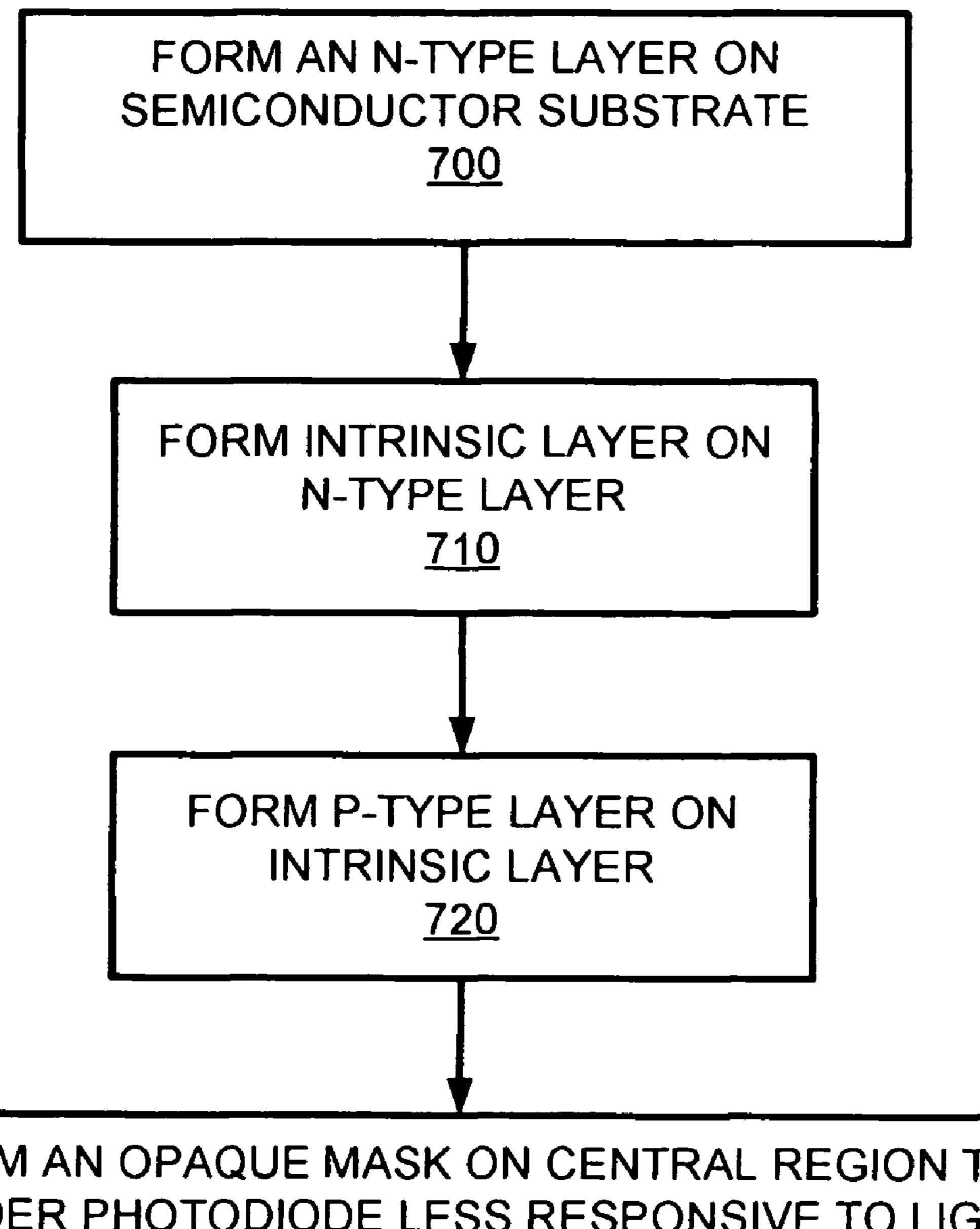
FORM AN OPAQUE MASK ON CENTRAL REGION TO RENDER PHOTODIODE LESS RESPONSIVE TO LIGHT ON CENTRAL REGION THAN TO LIGHT ON PERIPHERAL REGION
