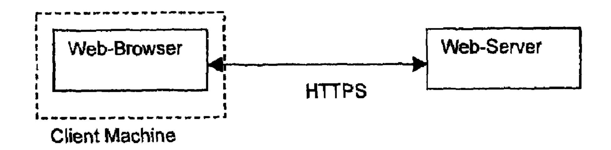
Figure 1: Secure Interaction Between a Web-Browser and a Web-Server
