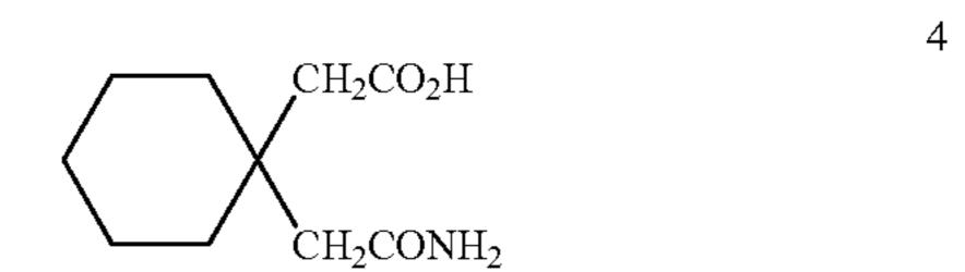
aging the resultant mixture; heating the mixture to a temperature in a range of 80 to 100 degrees C.; extracting with nonpolar solvent and distilling under reduced pressure to obtain gabalactam.
