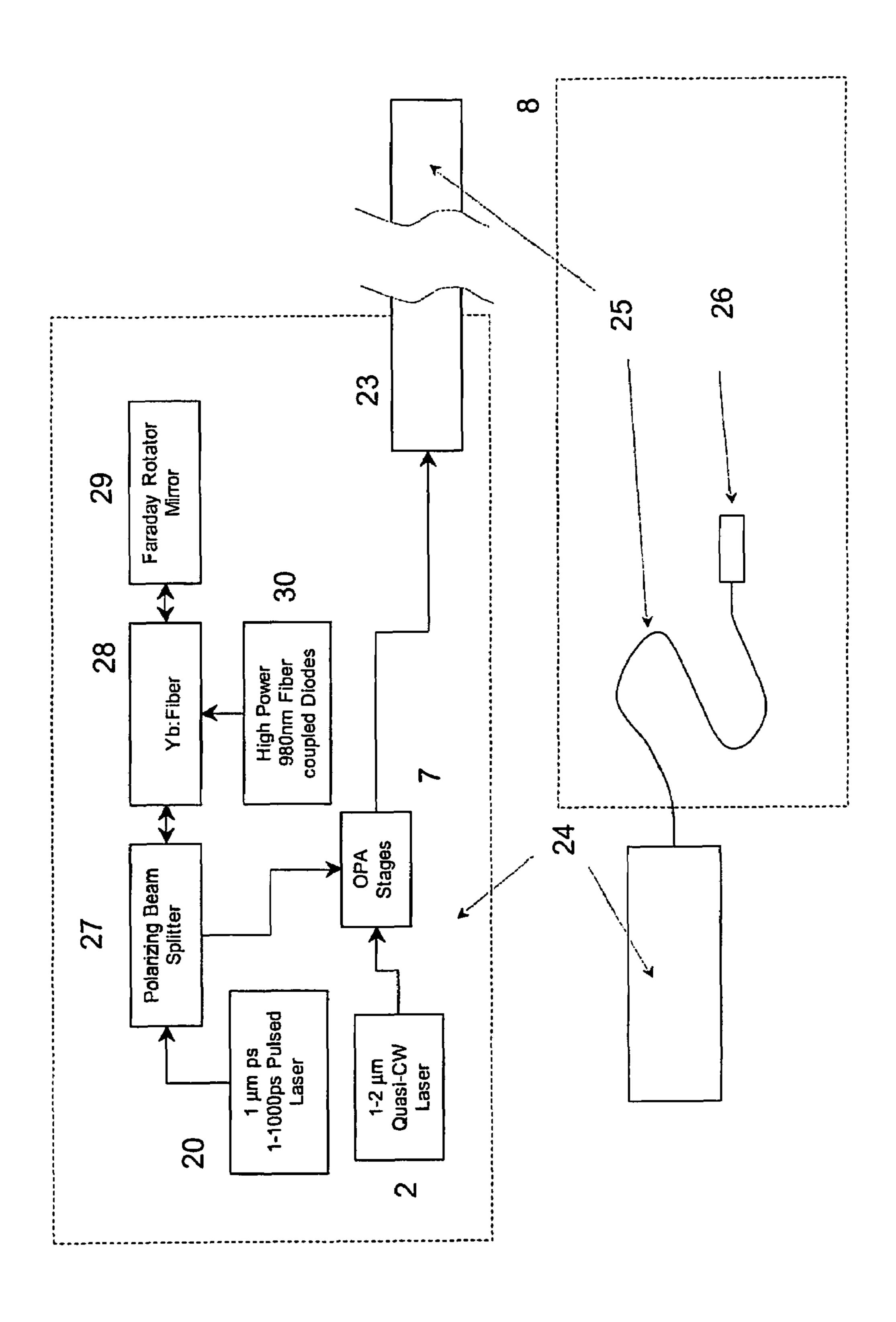
Polarization Maintaining Large Core Y b doped Fiber Amplifier  $\infty$ 23 1.6 μm Quasi-CW Laser 5 2 High Power Pump Diodes 1 µm ps 1-1000ps Pulsed Laser
