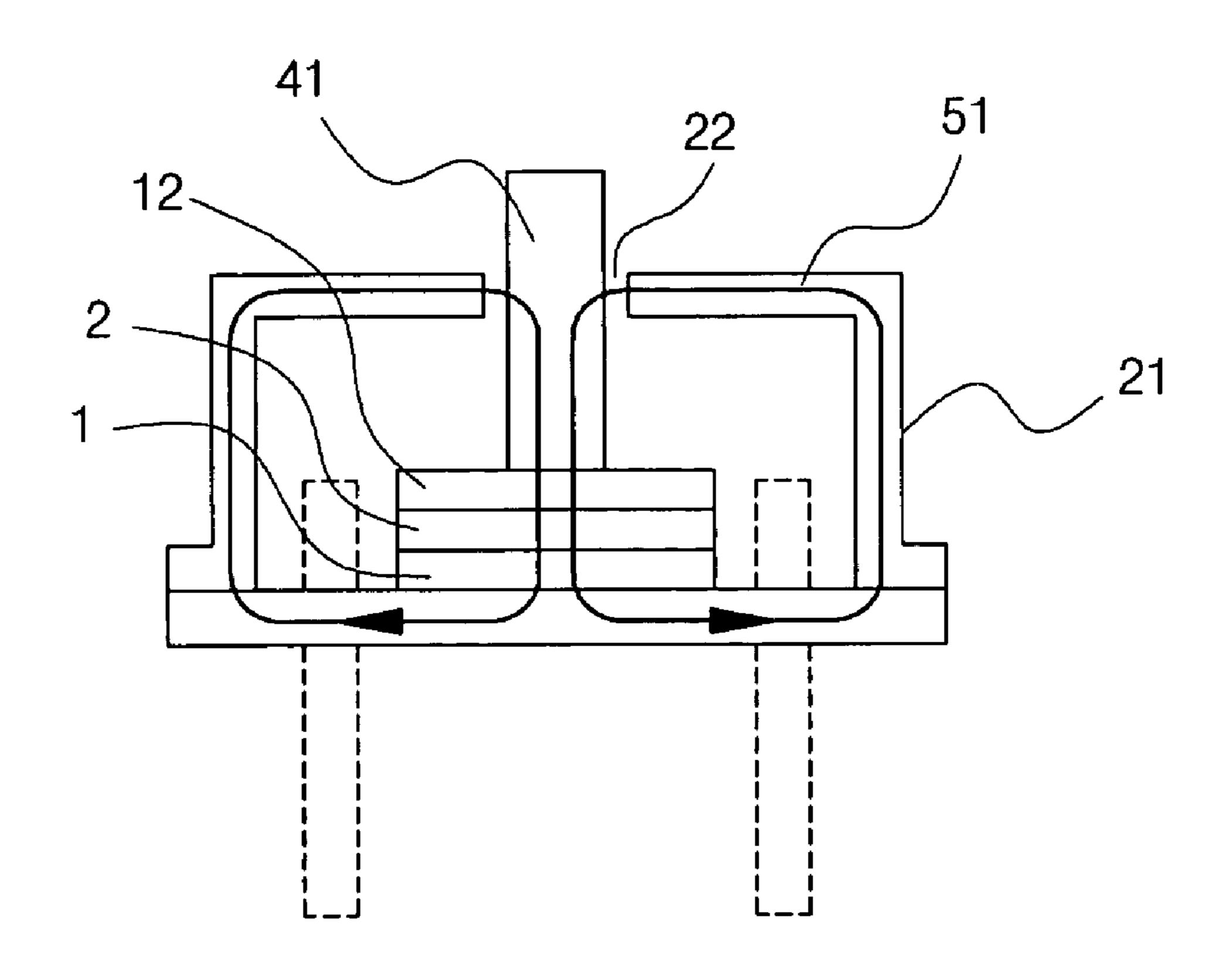
SURFACE ACOUSTIC WAVE LINEAR MOTOR, SURFACE ACOUSTIC WAVE LINEAR MOTOR PACKAGE, AND LENS ACTUATOR ADOPTING THE SURFACE ACOUSTIC WAVE LINEAR MOTOR PACKAGE
