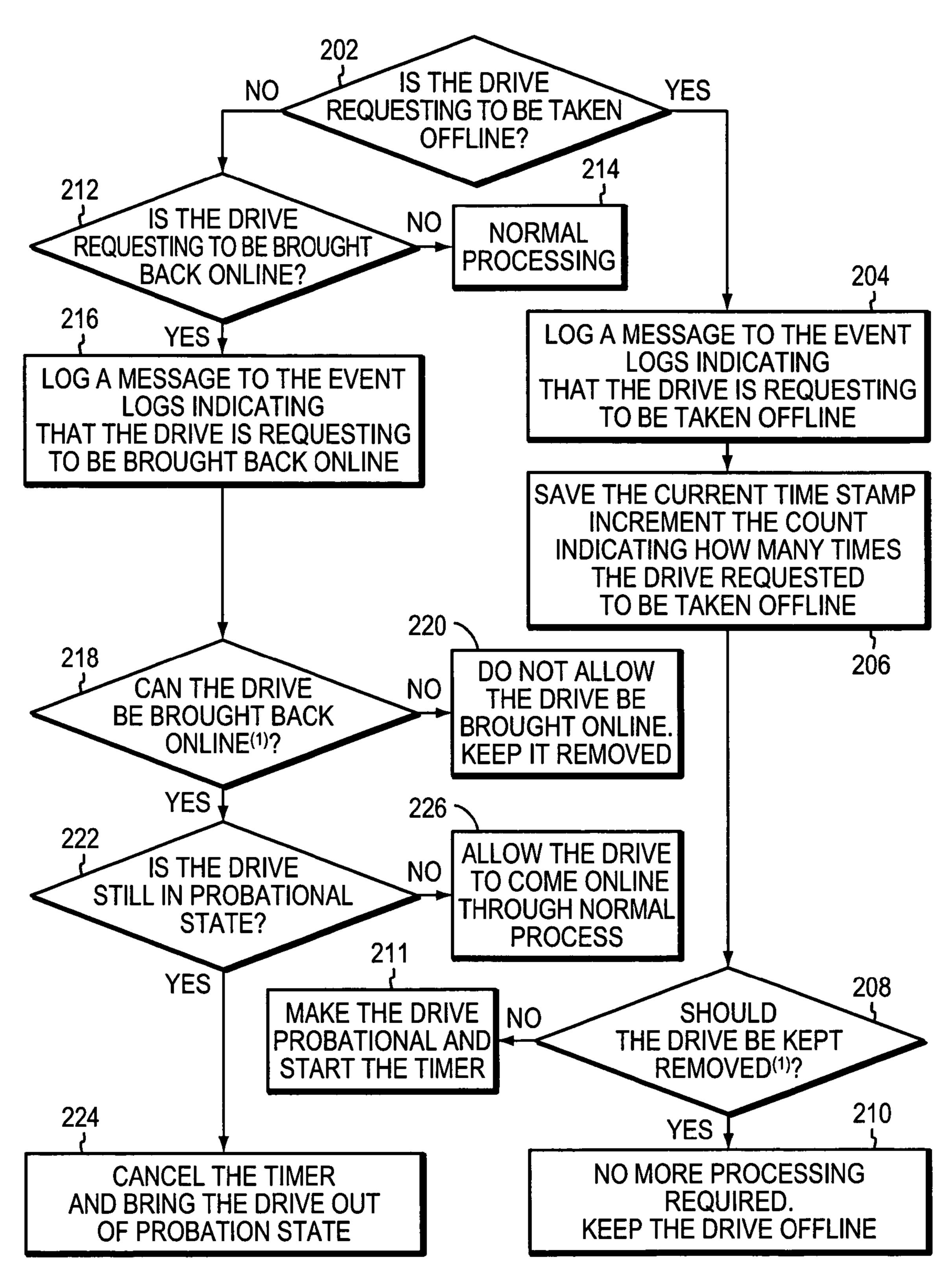
(1) - IF A DRIVE IS REQUESTING TO BE BYPASSED MORE THAN ONCE IN 24 HOUR PERIOD, DECLARE THIS AS UNSTABLE DRIVE AND KEEP THE DRIVE REMOVED
