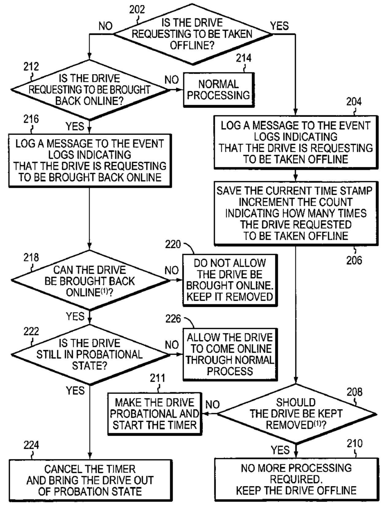
(1) - IF A DRIVE IS REQUESTING TO BE BYPASSED MORE THAN ONCE IN 24 HOUR PERIOD, DECLARE THIS AS UNSTABLE DRIVE AND KEEP THE DRIVE REMOVED
