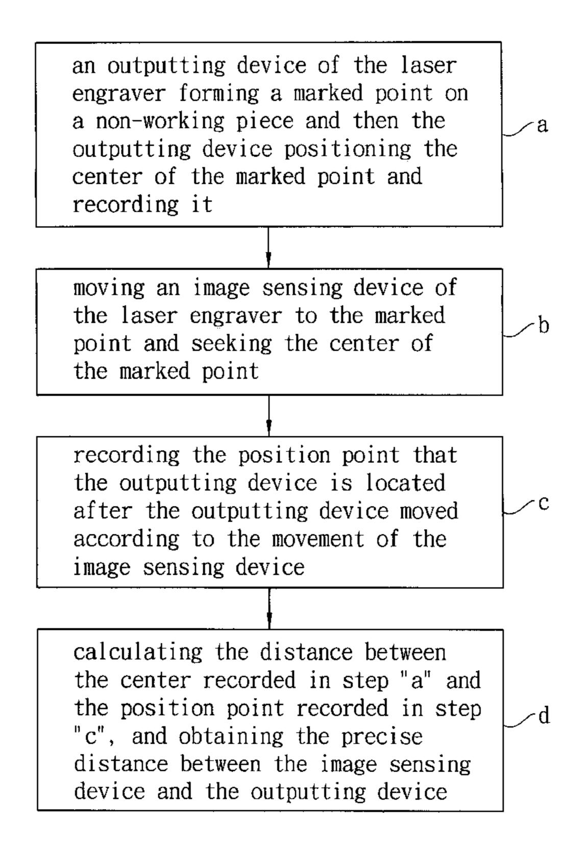
an outputting device of the laser engraver forming a marked point on a non-working piece and then the outputting device positioning the center of the marked point and recording it
