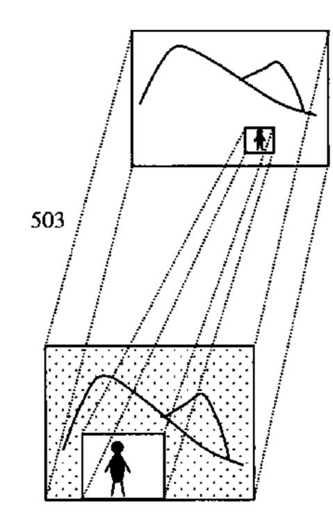
Picture-in-Picture full field of view decimated window & zoom window of moving target
