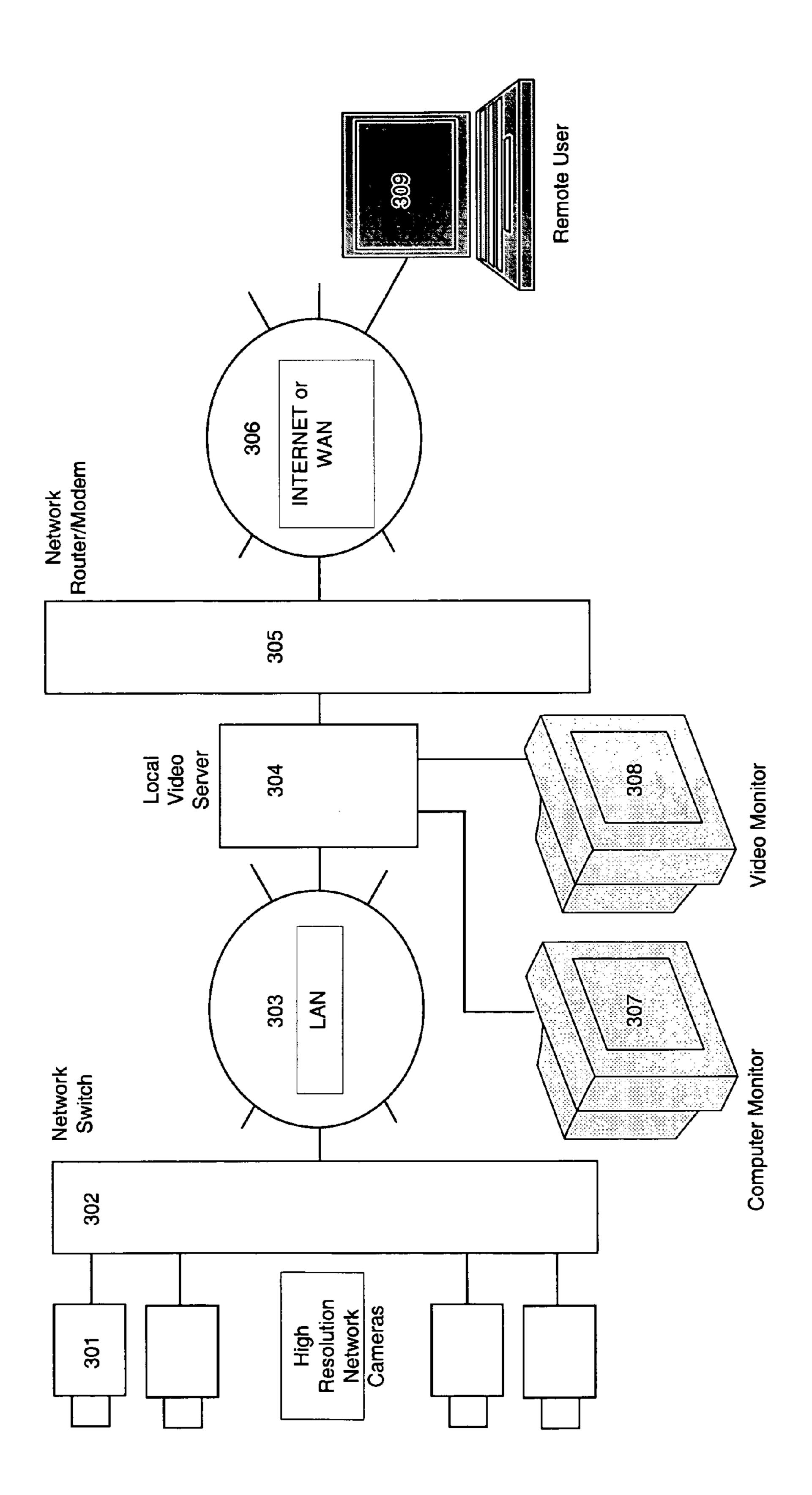
Figure 3. Multi-camera surveillance system
