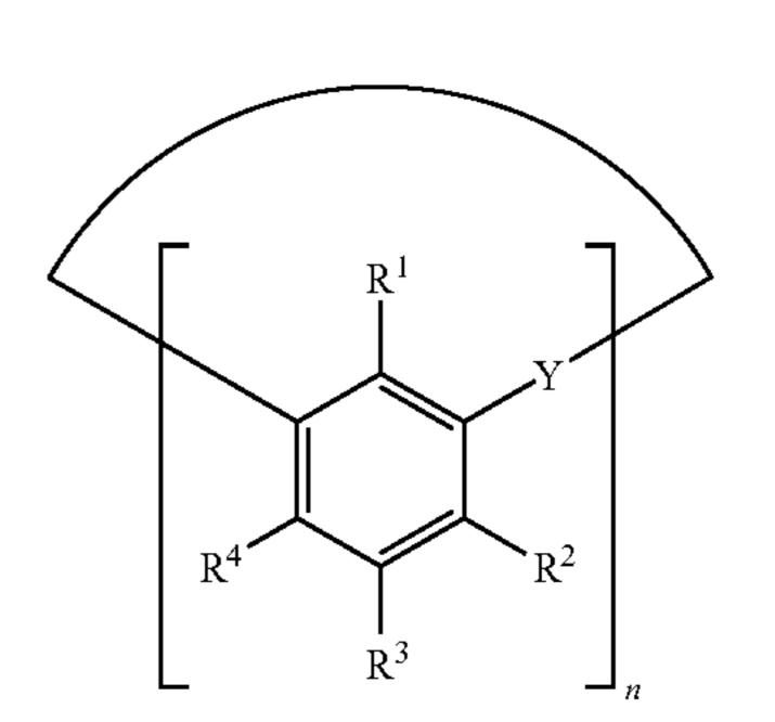
wherein in formula (III): Y is a divalent bridging group, at least one of said bridging groups being a sulfur atom; R<sup>3</sup> is hydrogen or a hydrocarbyl group; either R<sup>1</sup> is hydroxyl and R<sup>2</sup> and R<sup>4</sup> are independently either hydrogen or hydrocarbyl, or R<sup>2</sup> and R<sup>4</sup> are hydroxyl and R<sup>1</sup> is either hydrogen or hydrocarbyl; and n is a number having a value of at least 4.
