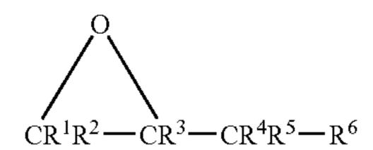
wherein R<sup>1</sup>, R<sup>2</sup>, R<sup>3</sup>, R<sup>4</sup> and R<sup>5</sup> are each, independently, hydrogen, or substituted or unsubstituted alkyl, or R<sup>2</sup> and R<sup>4</sup> may be taken together to form a 5-7 membered ring, and
