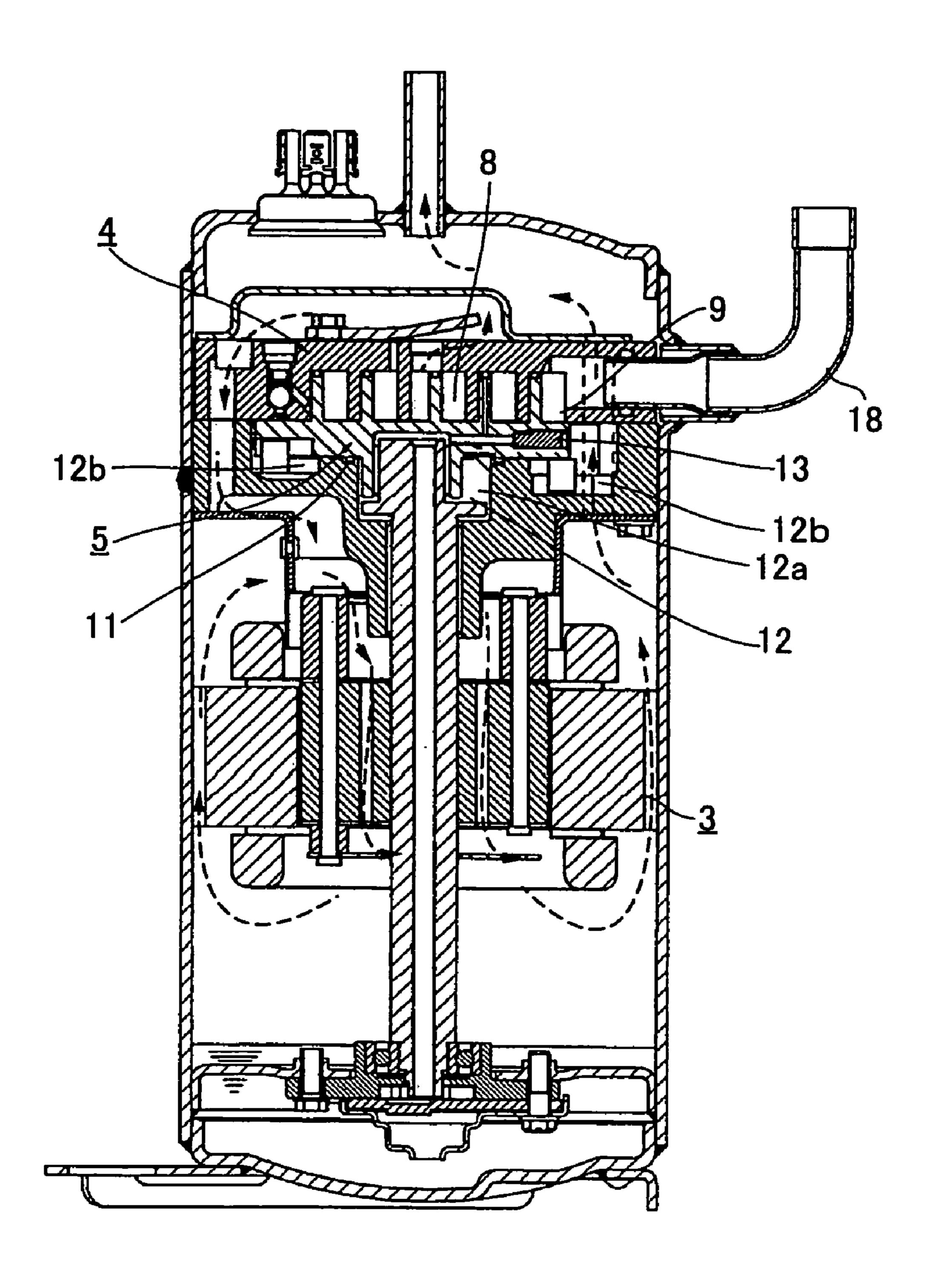
SCROLL COMPRESSOR WITH CERTAIN PRESSURE RATIO BETWEEN DISCHARGE PRESSURE AND SUCTION PRESSURE AND WITH CERTAIN RATIO OF DIAMETER OF ORBITING MIRROR PLATE AND OUTER DIAMETER OF THE ANNULAR SEAL
