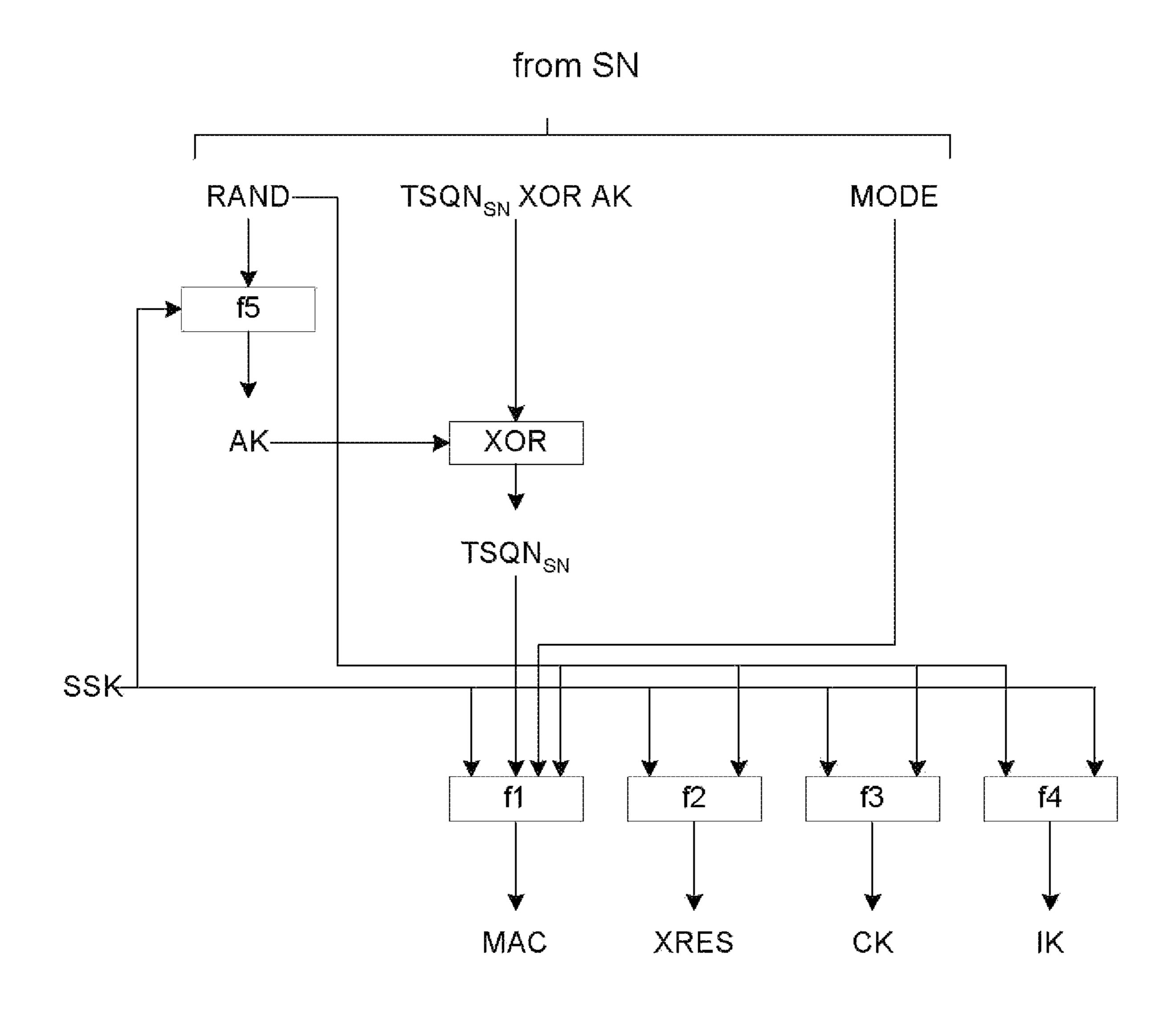
Verify MAC = XMAC Verify TSQN<sub>SN</sub> > TSQN<sub>USIM/MS</sub>
