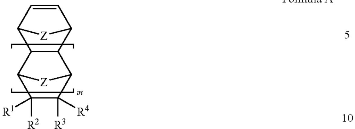
where for Formula A, m is an integer from 0 to 5; and Z represents — $(CH_2)_p$ —, where p is equal to 1; and where one of  $R_1$  to  $R_4$  is independently a fluorinated carbinol pendent 15 group represented by the following formula:
