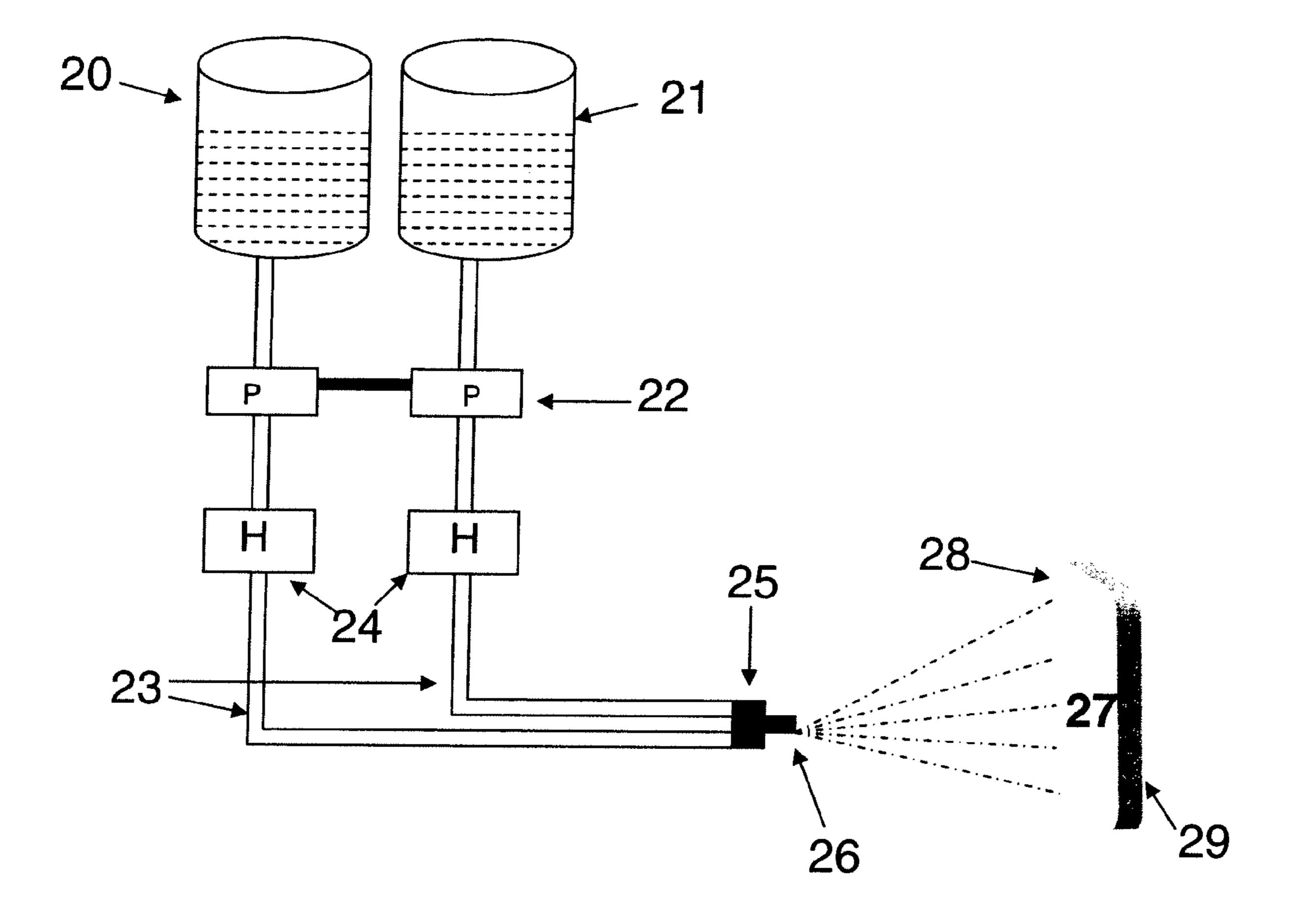
Figure 2. Plural Component Spray Equipment for Ballistic Substrate Coating
