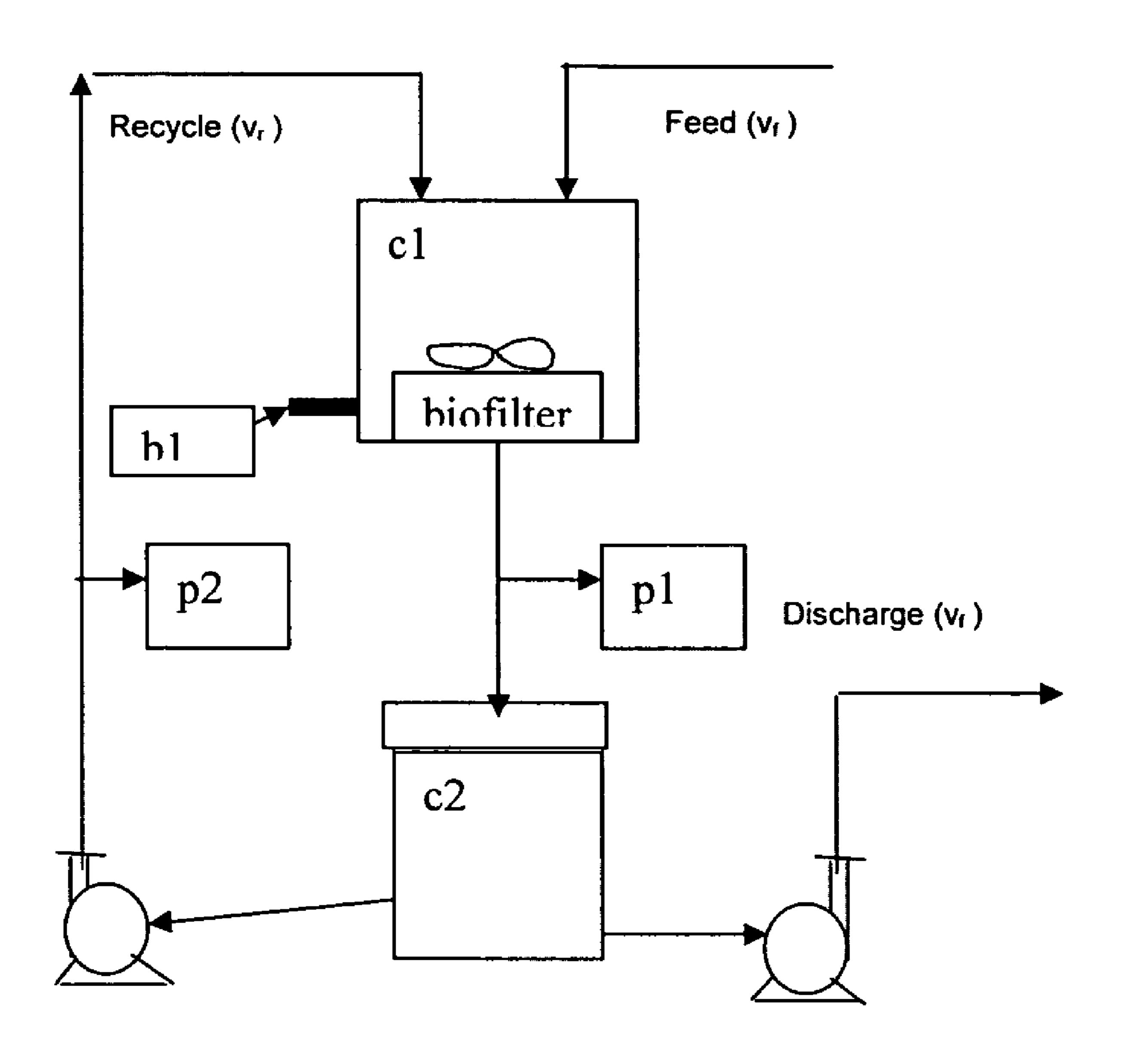
Figure 1: Schematics of biofilter operation
