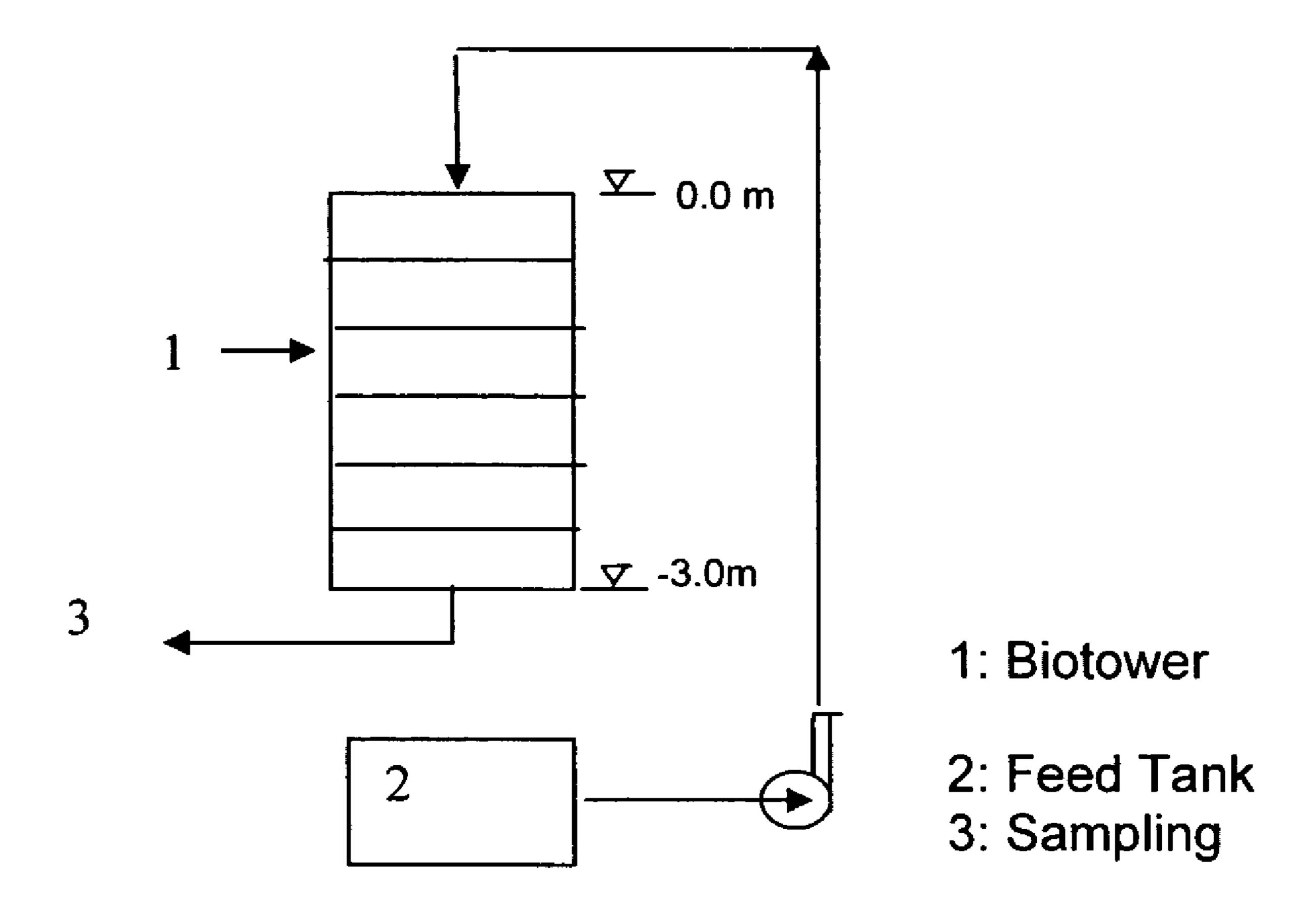
Figure 3: Schematics of a Biotower
