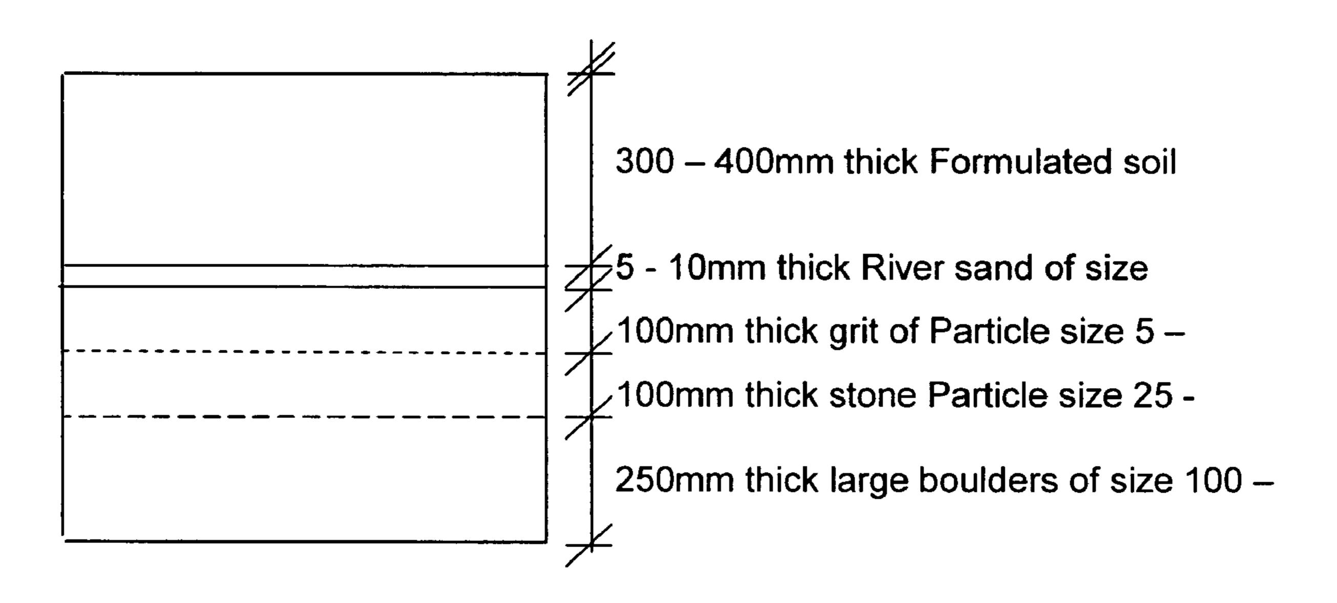
Fig 2: Biofilter Filling Details
