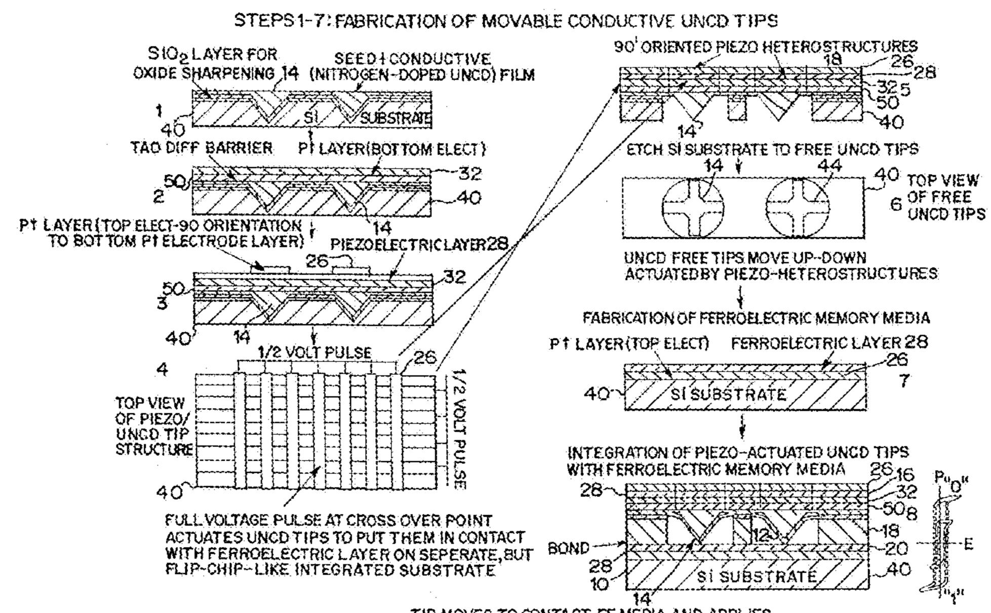
TIP MOVES TO CONTACT FE MEDIA AND APPLIES VOLTAGE TO POLARIZE MEDIA AND IMPRINT INFORMATION
