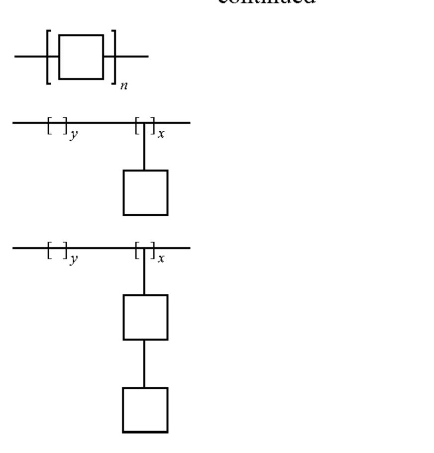
in which the continuous line is the main chain of the siloxane polymer and the squares represent the groups capable of establishing hydrogen interactions.
