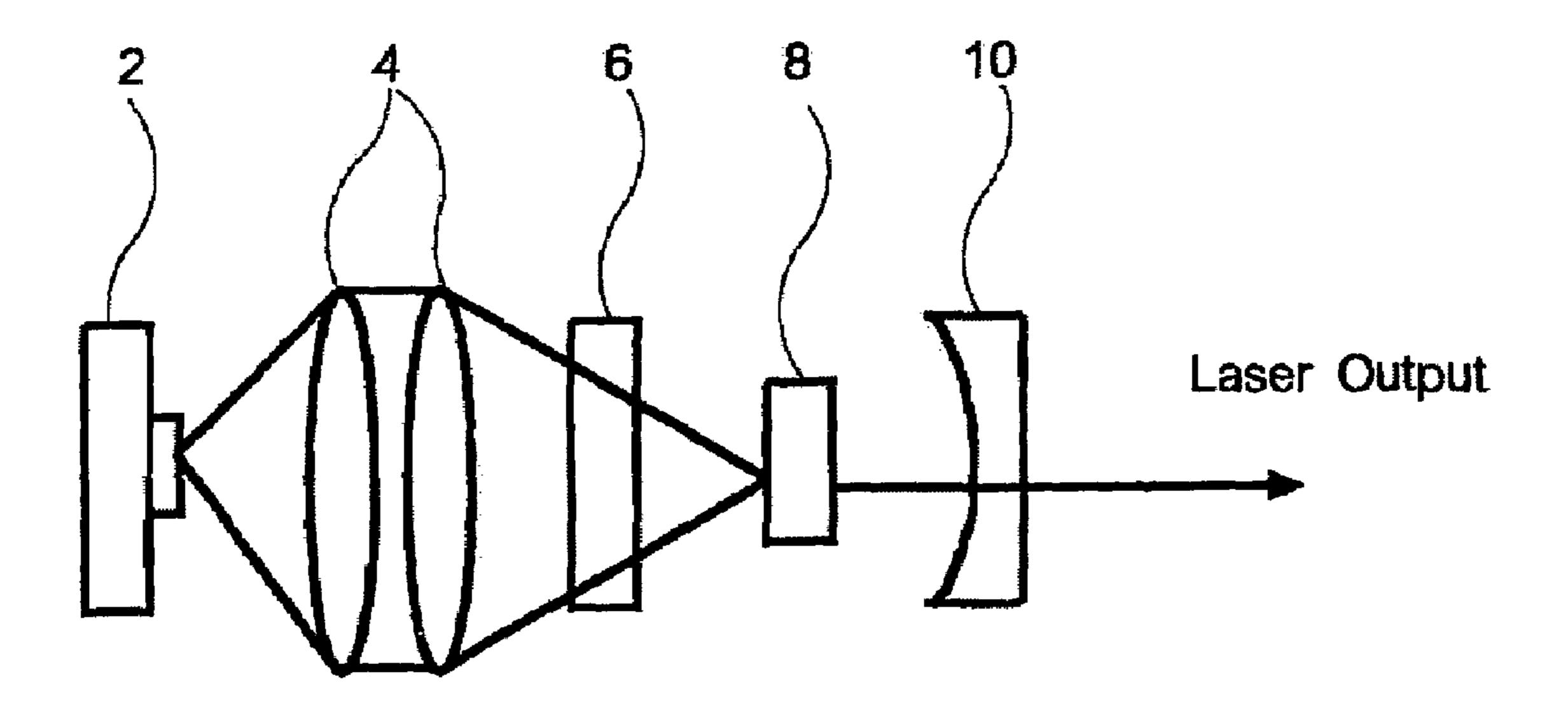
8: Nd:Lu2O3 10: OC:T-3% 2: 1W LaserDiode 4: Lense 6: HR R=50mm Ceramics f=8mm (808nm)
