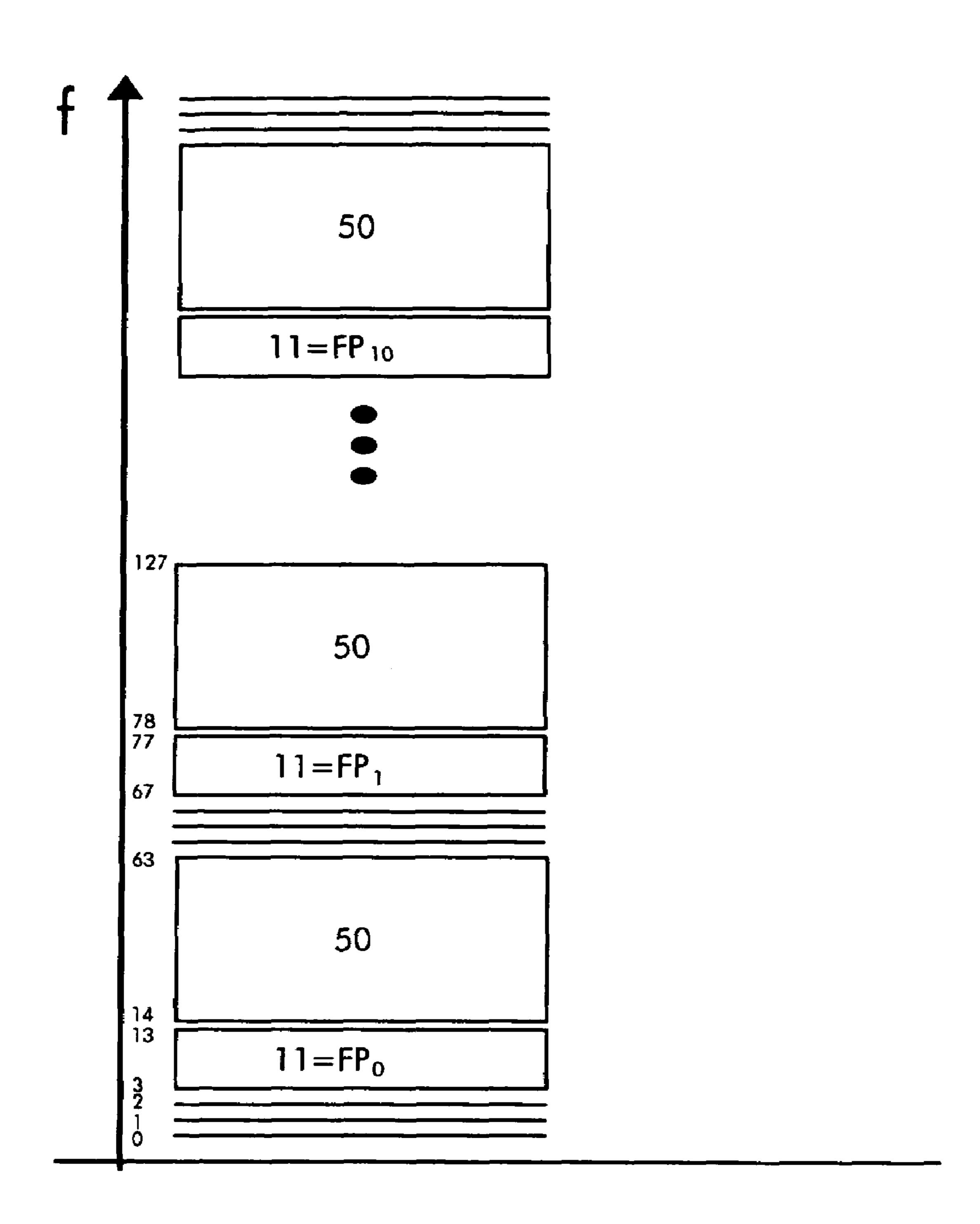
METHOD FOR DISTRIBUTING DATA ON AN OFDM TIME-FREQUENCY GRID ALLOWING FOR COORDINATION OF INTERFERENCES AND ADAPTIVE SUBCARRIER FREQUENCY ALLOCATION, A BASE TRANSCEIVER STATION, A BASE STATION CONTROLLER AND A MOBILE NETWORK THEREFOR
