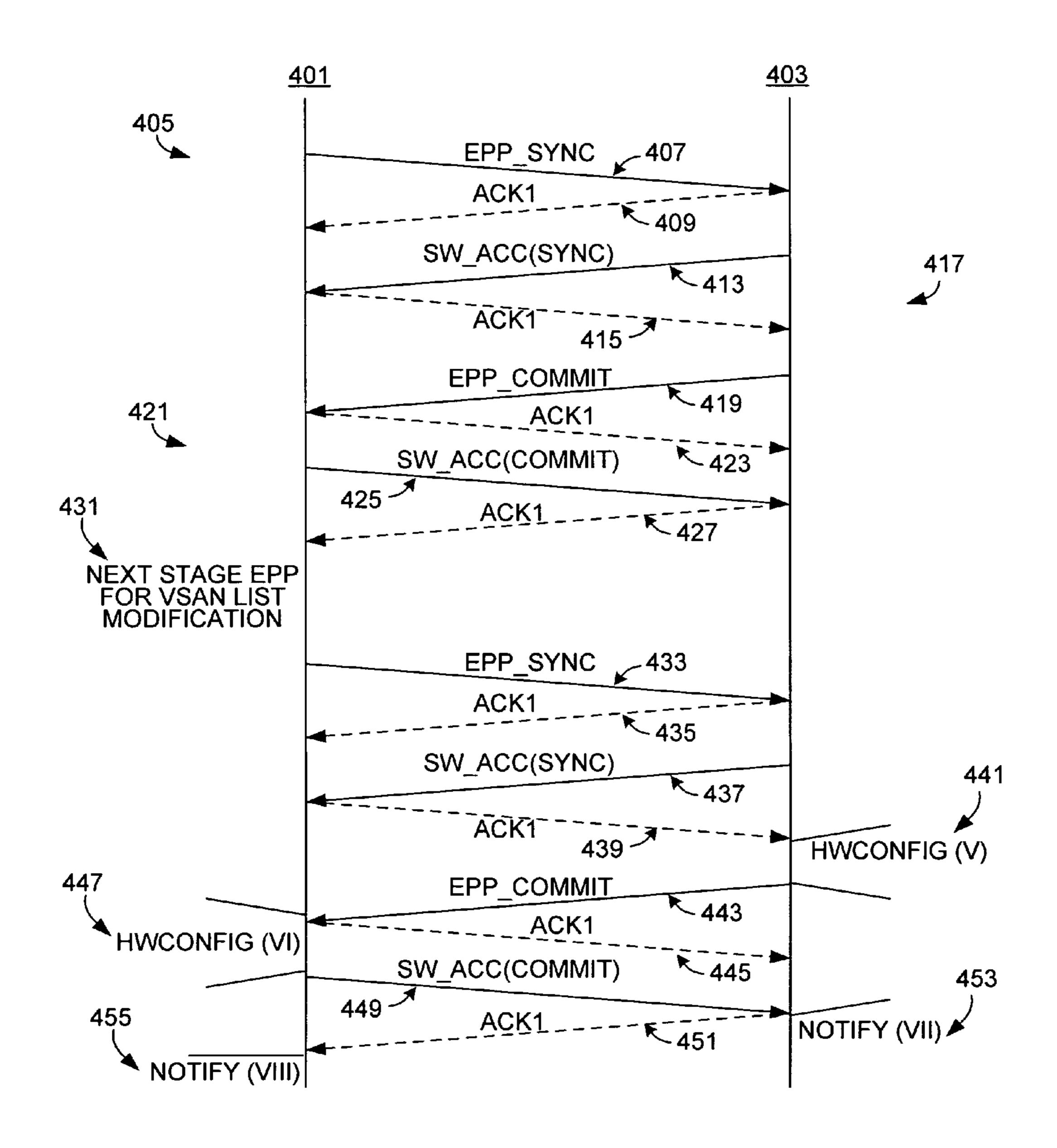
EPP graceful port shutdown exchange for VSAN removal for a TE Port (Single Physical Link or Port Channel)
