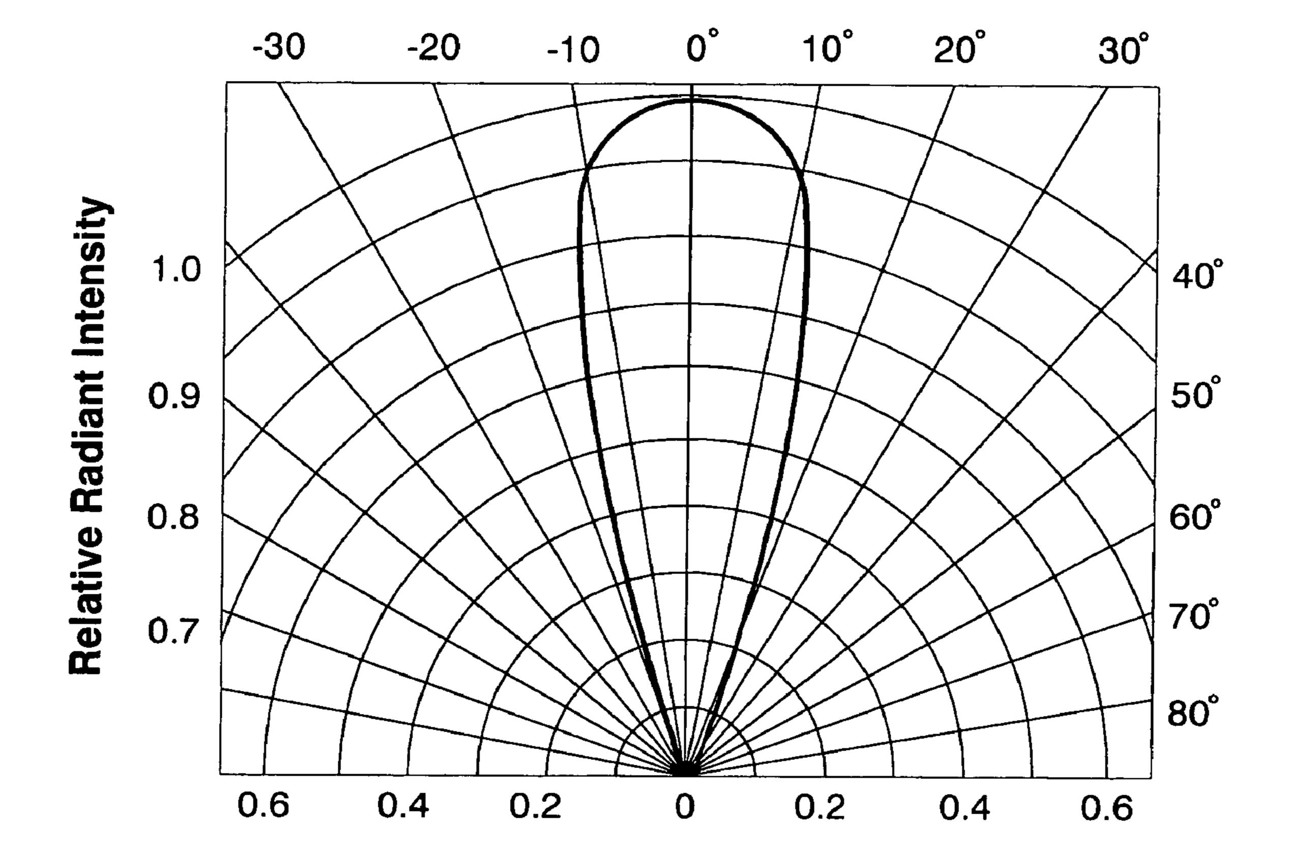
Relative Radiant Intensity vs. Angular Displacement Fig. 4
