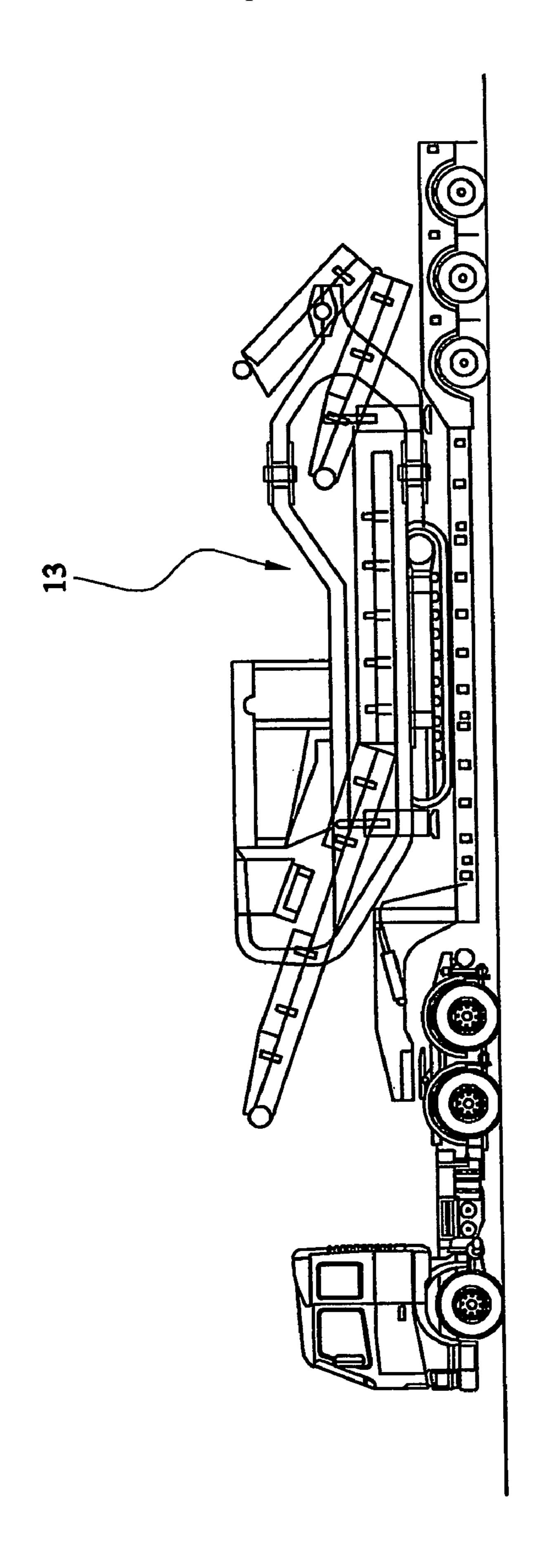
DISCHARGE (3) SECTION IN TRANSPORT POSITION
