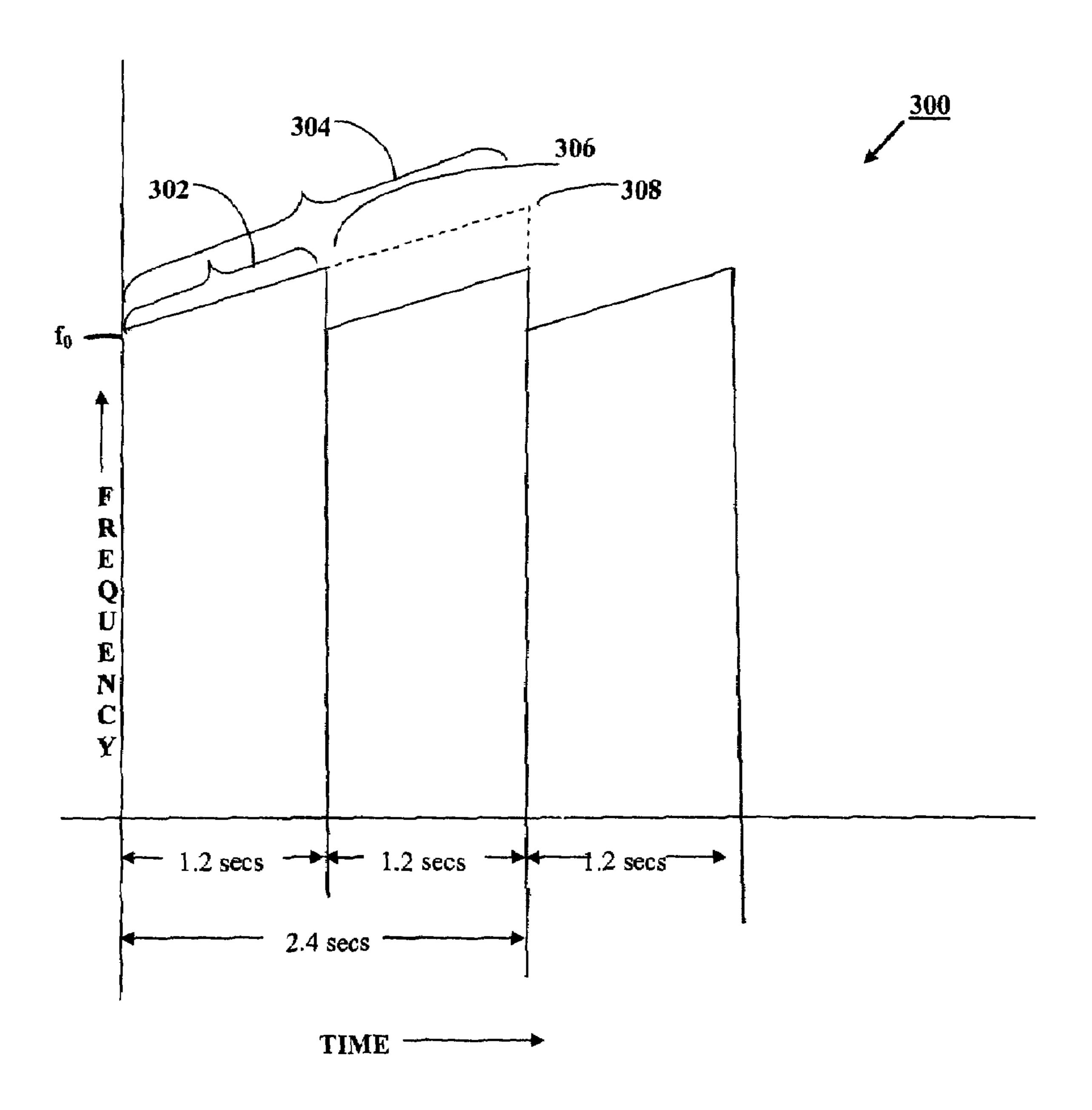
FIG. 3 TEMPERATURE RAMP COMPENSATION
